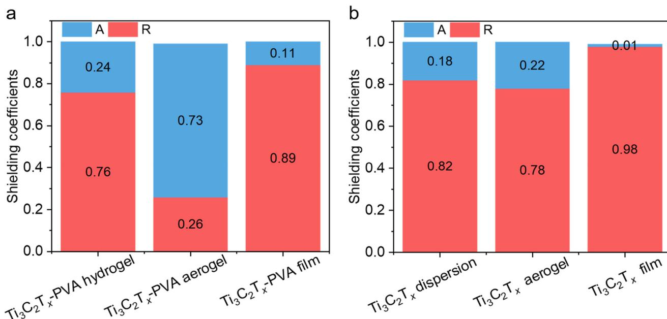
Fig. 5 Absorption coefficient ( $A$ ) and reflection coefficient ( $R$ ) of the (a)  $Ti_3C_2T_x$ -PVA-based hydrogel, aerogel, and film and (b)  $Ti_3C_2T_x$ -based dispersion, aerogel, and film at a fixed  $Ti_3C_2T_x$  areal density ( $20 \text{ mg cm}^{-2}$ ).
