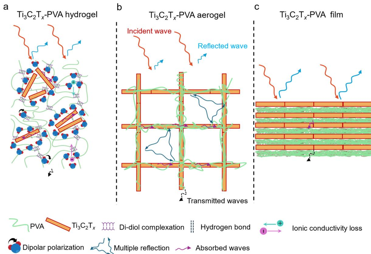
**Fig. 6** Schematic illustrations of the EMI shielding mechanism in (a)  $\text{Ti}_3\text{C}_2\text{T}_x$ -PVA hydrogels, (b)  $\text{Ti}_3\text{C}_2\text{T}_x$ -PVA aerogels, and (c)  $\text{Ti}_3\text{C}_2\text{T}_x$ -PVA compact films. The diagrams highlight the key factors contributing to EMI shielding performance reflection, absorption, and internal multiple reflections and their respective roles in attenuating electromagnetic waves.
