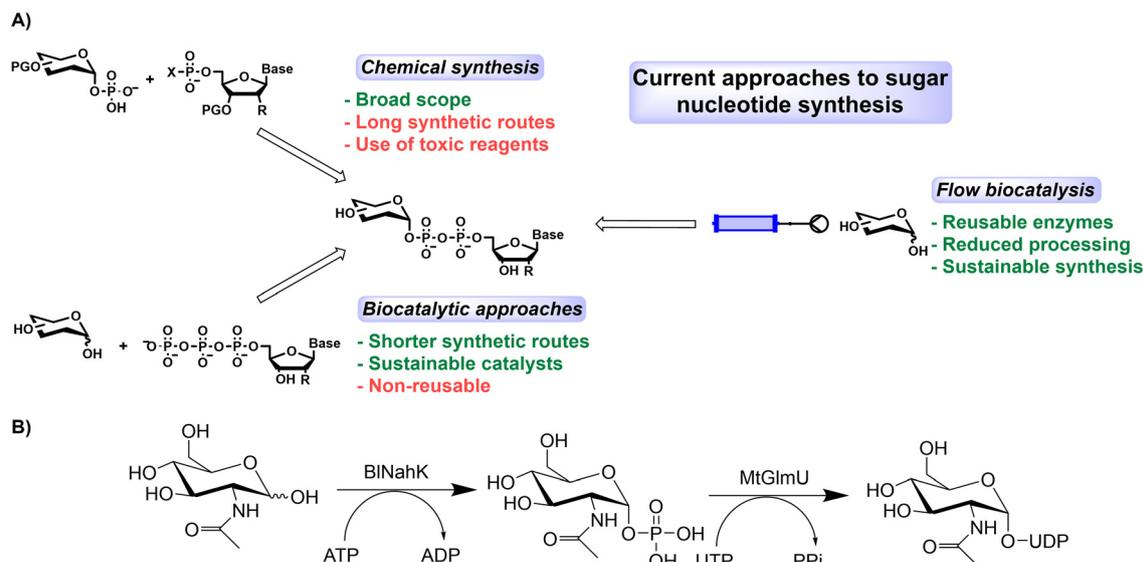
**Fig. 1** A) Current approaches to sugar nucleotide synthesis and B) biotransformation of GlcNAc to UDP-GlcNAc utilising two enzymes, BINahK and MtGlmU. In soluble batch cascades a further enzyme (iPPase) is added to break down the inorganic phosphate (PPi) which has an inhibitory effect on the MtGlmU.<sup>30</sup>
