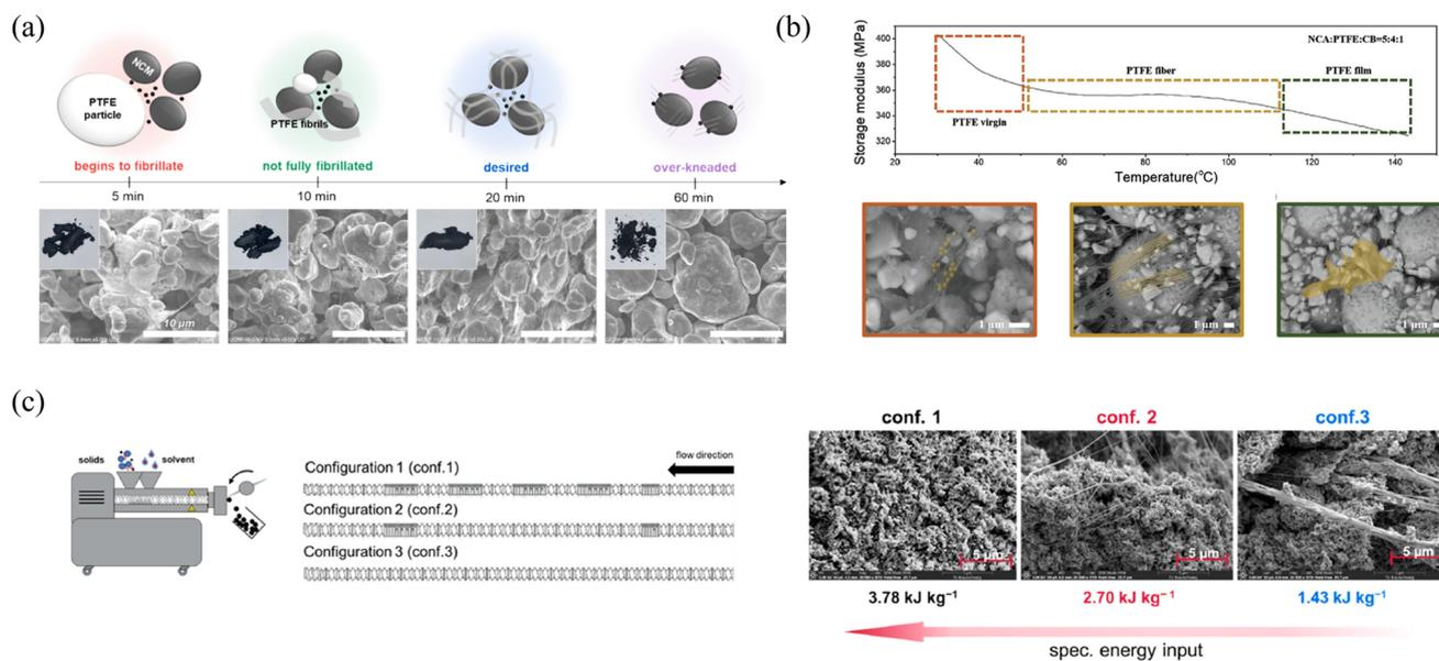
Fig. 8 Engineering of the PTFE fibrillization process (LIBs). Investigation of PTFE fibrillization behavior according to the (a) fibrillization process time, (b) fibrillization process temperature and (c) the number of kneading configurations. Reproduced with permission from ref. 83, 88 and 89. Copyright (2024) The Authors. Published by Elsevier B.V., copyright (2024) Wiley-VCH GmbH and copyright (2023) The Authors. Licensee MDPI, Basel, Switzerland.
