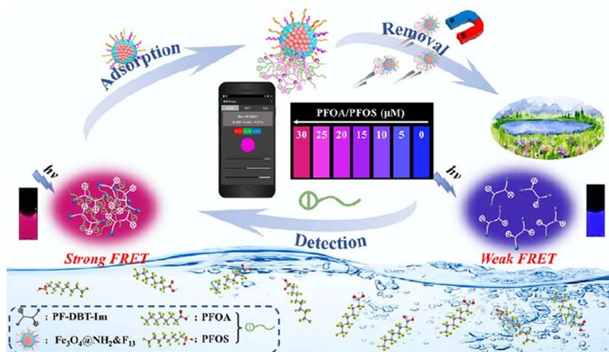
Fig. 1 Schematic illustration of the two-in-one platform for PFOA/PFOS detection and removal.<sup>19</sup>
