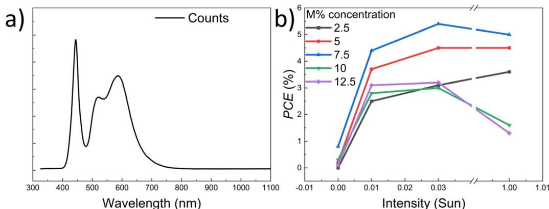
Fig. 4 (a) Spectrum of the LED used to test indoor PV performance and (b) the corresponding PCE under different light intensities for FASI with different mol% concentration of MASnCl<sub>3</sub>.
