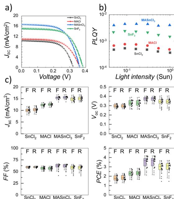
Fig. 3 Comparison of the performance of FASnI<sub>3</sub> devices printed with the four additives studied, SnCl<sub>2</sub>, MACl, MASnCl<sub>3</sub>, SnF<sub>2</sub>. (a) JV scans; (b) light-intensity-dependent photoluminescence quantum yield of each sample (full device stack); (c) JV performance distribution (F for forward and R for reverse scans) of each sample.
