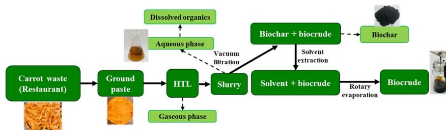
Fig. 2 Flow chart of different steps involved in the conversion of food waste into biocrude through hydrothermal liquefaction (HTL).
