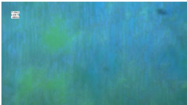
Fig. 12 POM image of DIO in Sm<sub>Z</sub>A phase right above threshold for magnetic FT. Periodic striations perpendicular to rubbing direction are observed (not seen in N phase).
