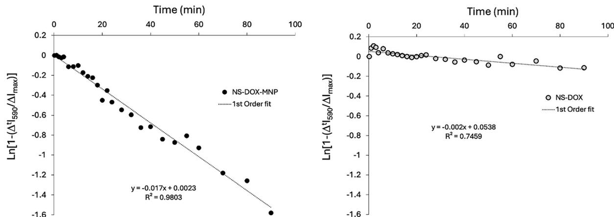
Fig. 7 1st order kinetic plots for NS-DOX-MNP sample (left) and the NS-DOX sample (right).  $\Delta I_{590}^t$  is the change in fluorescent intensity at 590 nm =  $(I_{590}^t - I_{800}^t) - (I_{590}^0 - I_{800}^0)$ , where  $I_{590}^t$  and  $I_{800}^t$  are the fluorescent intensity for time  $t$  at 590 nm and 800 nm respectively and  $I_{590}^0$  and  $I_{800}^0$  are the fluorescent intensity for time = 0 at 590 nm and 800 nm respectively.
