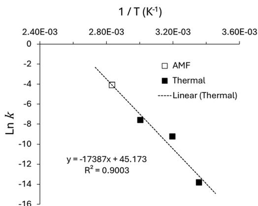
**Fig. 9** Arrhenius plot for the thermal release data showing the inverse linear dependence of the rate constant for the diffusion of DOX from inside the NS-DOX-MNP samples, on the temperature of the system ( $k$  is the 1st order rate constant ( $\text{min}^{-1}$ ) and  $T$  is temperature in Kelvin). The linear fit is for the thermal release data only. The AMF data point shows the predicted temperature of the magnetic release (AMF) rate constant based on the linear fit.
