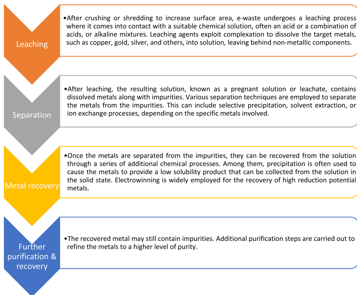
Fig. 5 Main phases of a typical hydrometallurgical process for e-waste treatment.
