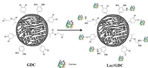
Fig. 16 Schematic illustration of immobilization of laccase on GDC beads.<sup>132</sup> Copyright Springer, 2020.
