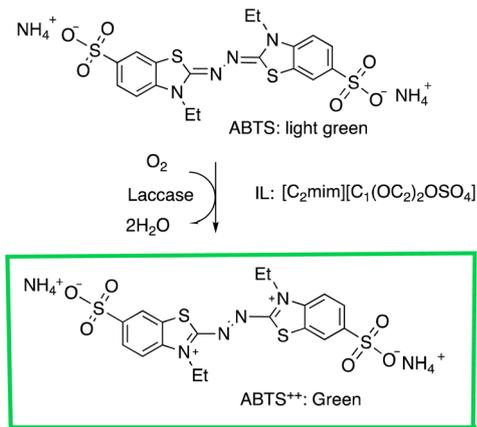
Fig. 7 Additive effect of an IL ([C<sub>2</sub>mim][C<sub>1</sub>(OC<sub>2</sub>)<sub>2</sub>OSO<sub>3</sub>]) on the laccase-mediated oxidation of ABTS.<sup>91</sup>
