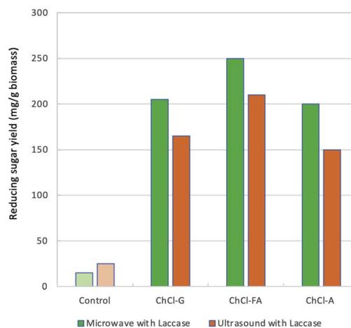
Fig. 28 Increased saccharification efficiency in the combinatorial method of pretreatment of laccase and DES.<sup>181</sup> Copyright Elsevier, 2023.
