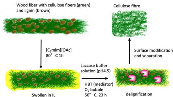
Fig. 25 Preparation of cellulose fibre using an IL and a subsequent laccase-catalysed reaction.<sup>63</sup> Copyright Elsevier, 2012.
