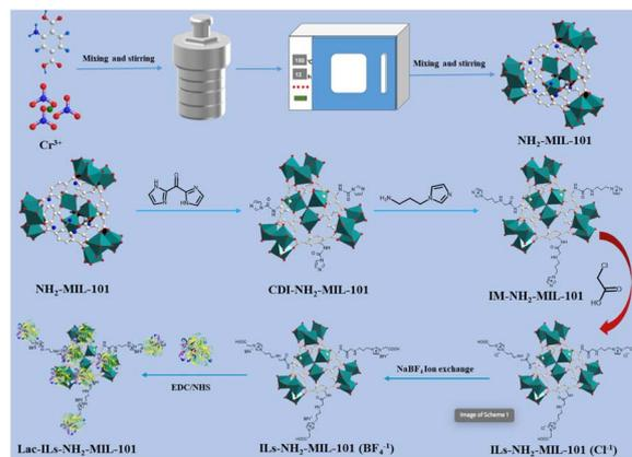
Fig. 18 A schematic diagram illustrating the covalent immobilization of laccase on ILs-NH<sub>2</sub>-MIL-101.<sup>140</sup> Copyright Elsevier, 2023.
