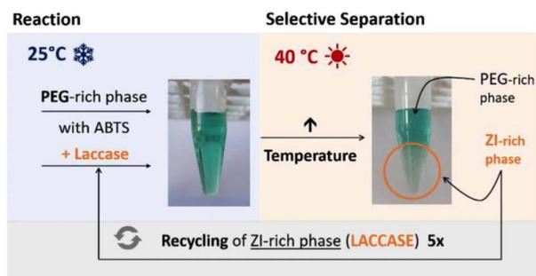
Fig. 10 Oxidation of ABTS using laccase in a mixed solvent of PEG and IL, N5,5,5C3S. Selective separation from the reaction product and catalyst by changes in the temperature.<sup>105</sup> Copyright RSC, 2018.
