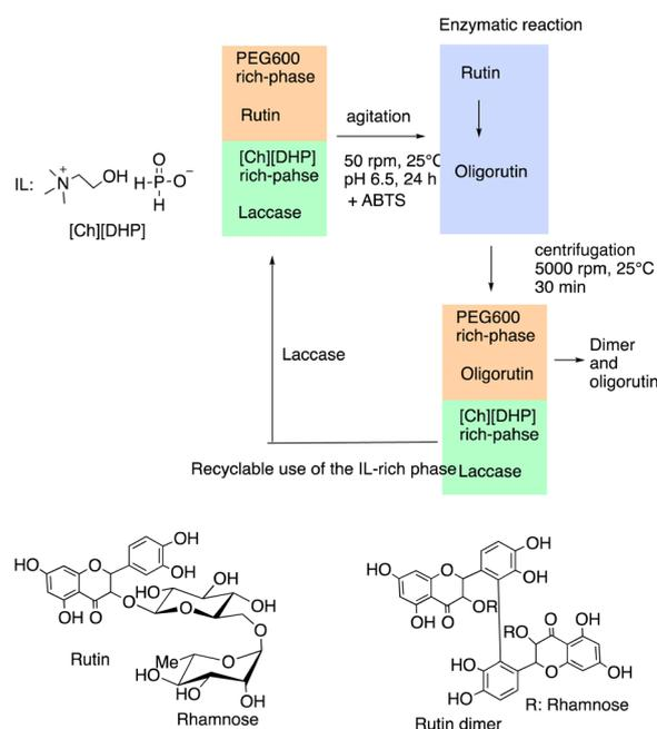
Fig. 32 Laccase-catalysed system for the dimerization of rutin.<sup>208</sup>
