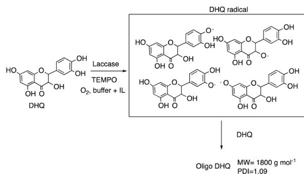
Fig. 31 Polymerization of dihydroquercetin (DHQ) by laccase-catalysed oxidation.<sup>206</sup>
