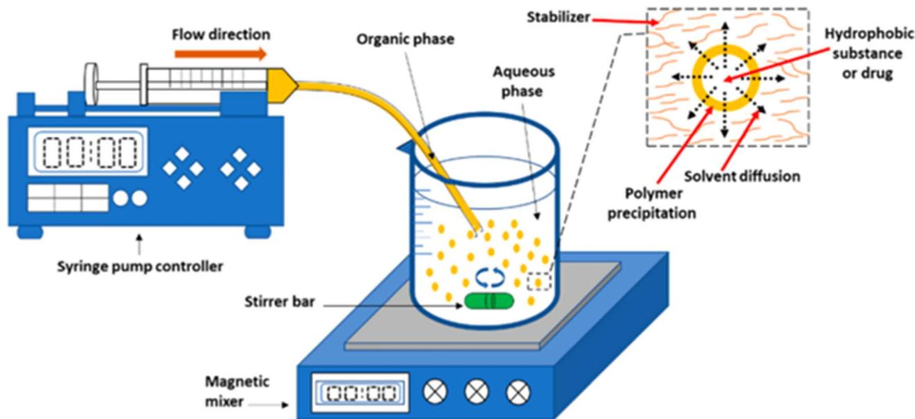
Fig. 9 Schematic representation of the anti-solvent nanoprecipitation method.<sup>99</sup> Adapted from an open-access article distributed under the terms of the Creative Commons Attribution License (CC BY).
