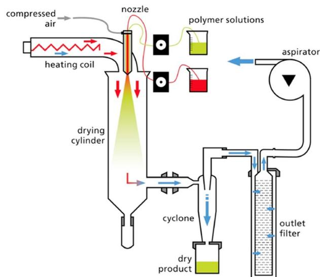
Fig. 11 Schematic of the spray drying process.<sup>105</sup> Reused with permission from the author.
