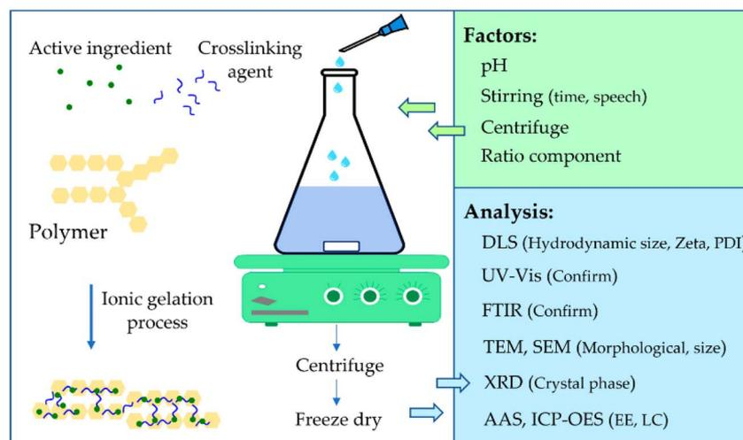
Fig. 10 Illustration of the ionotropic gelation method.<sup>102</sup> Adapted from an open-access article distributed under the terms of the Creative Commons Attribution License (CC BY).
