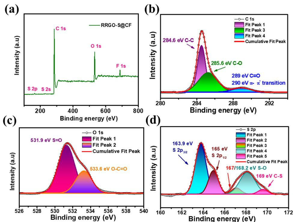
Fig. 2 XPS of the RRGO-S@CF electrode: (a) survey scan, (b) C 1s, (c) O 1s, (d) S 2p. The binding energy was calibrated with respect to the C 1s peak of 284.6 eV.
