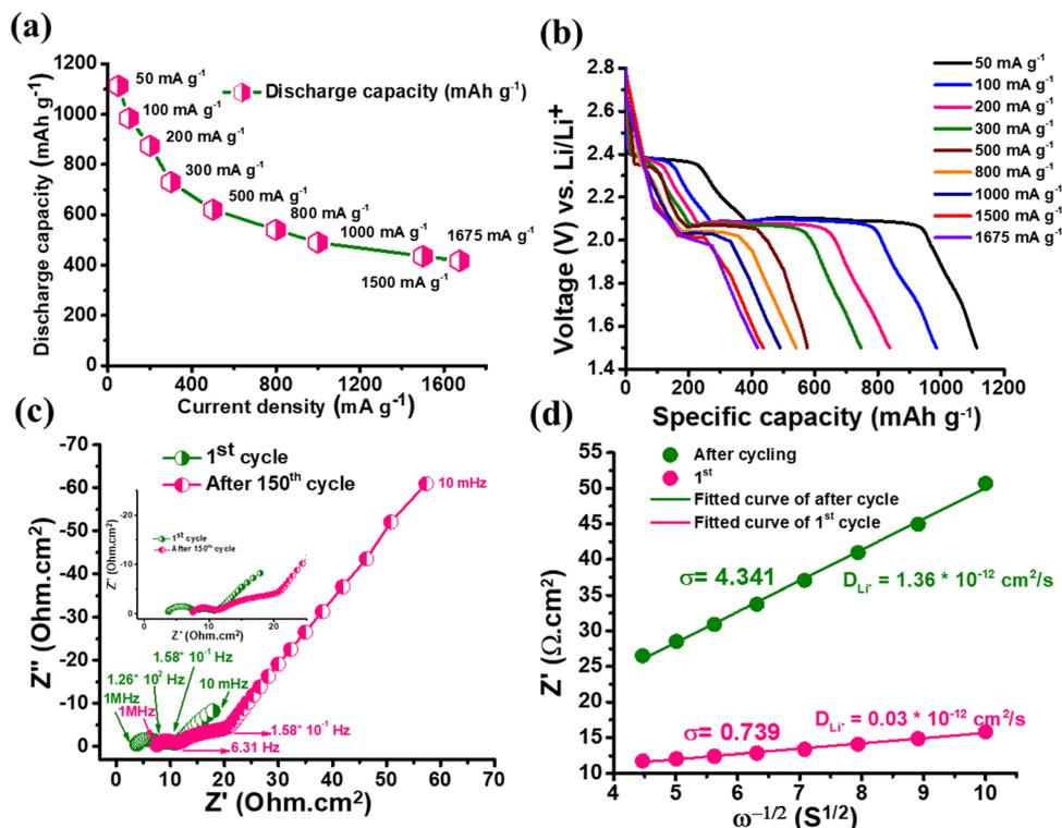
Fig. 5 (a) and (b) Rate capability plot at different current densities. (c) EIS spectra of RRGO-S@CF for the 1st and 150th cycle (cycling at  $200 \text{ mA g}^{-1}$ ) with their frequencies. (d) Plot of  $Z'$  vs.  $\omega^{-1/2}$  ( $\text{S}^{1/2}$ ) in the low-frequency region.
