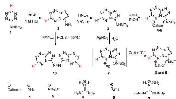
**Scheme 1** Preparation of energetic monosubstituted fused ring materials **4-6** and **8-10**
