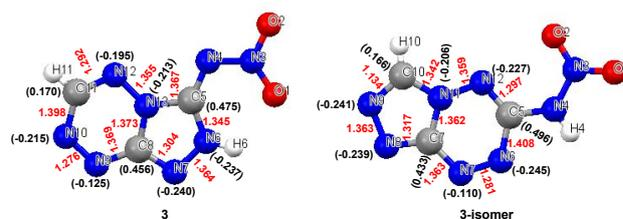
Fig. 3 Length of bonds (red numbers) and charge distribution (in parentheses) of **3** and **3-isomer**
