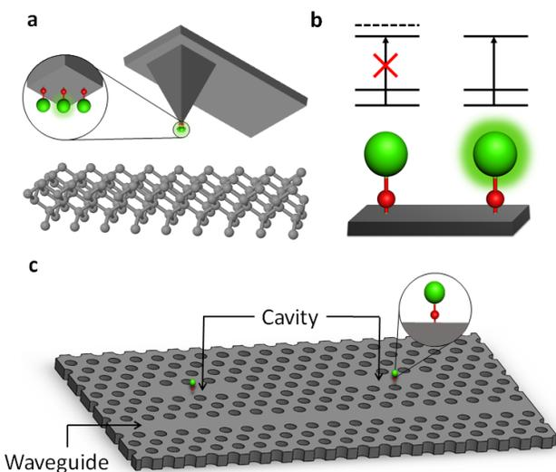
**Figure 6.** Applications of surface bound OCCs. (a) An AFM/STM tip can be functionalized with OCC centers, enabling precision quantum-enhance readout of local magnetic and electric fields through fluorescence. (b) Two OCCs in spatial proximity can provide the two qubit basis for a CNOT gate achieved through dipole blockade. (c) OCCs can be placed in a photonic waveguide, entangling two OCCs via photonic bus.
