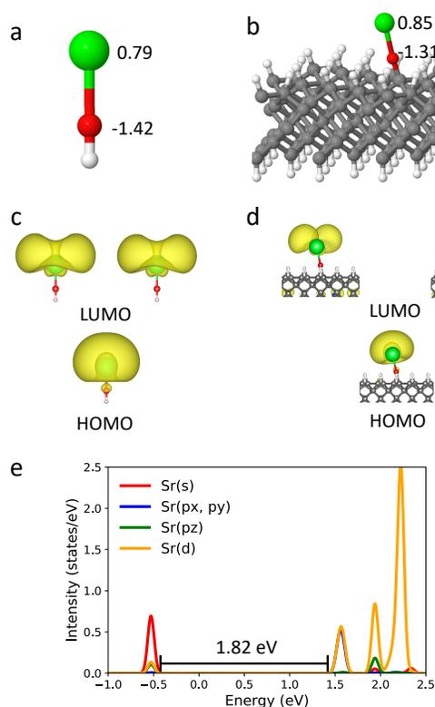
**Figure 2.** (a) (b) Optimized geometries of the gas-phase SrOH molecule and the SrO-group bound to the diamond surface. The green, red, gray and white colors represent the Sr, O, C and H atoms, respectively. The atomic charges on Sr and O from the Bader charge analysis are also shown. (c) (d) Electron density of the HOMO and LUMO of the SrOH molecule and the SrO supported on diamond. The isosurfaces are plotted with an isovalue of 0.001. (e) PDOS, indicating the excitation energy distance.
