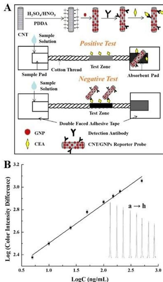
**Fig. 8** Other emerging paper-like hybrid microfluidic devices for cost-effective diagnostics. (A) Principle of using a cotton thread/paper hybrid device based on CNT/GNPs nanocomposite reporter probes for CEA detection. (B) Quantitative analysis of CEA in human serum samples using the cotton thread/paper hybrid device. Sample a to h: 5, 10, 25, 50, 100, 150, 200, and 500 ng/mL. Reprinted with permission from Ref. <sup>146</sup>. Copyright 2017 Elsevier.
