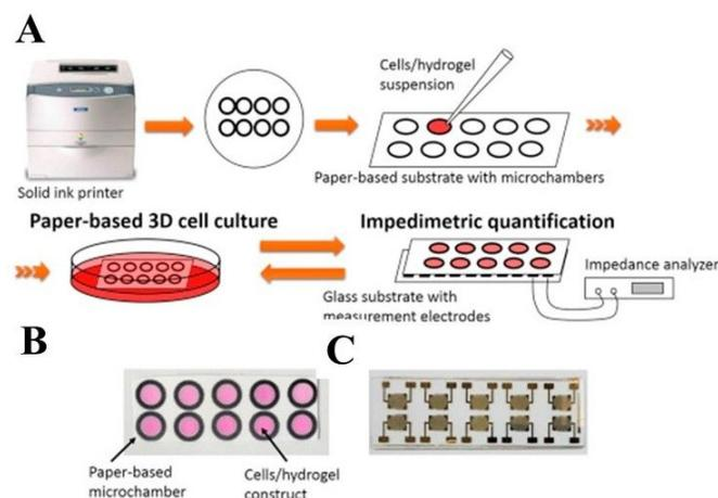
**Fig. 7** Paper/polymer hybrid microfluidic devices for 3D cell culture. The procedure of the impedimetric quantification of cell proliferation using the paper/glass hybrid microchambers. (A) Illustration of cell seeding, culture, and measurement processes. (B) Photograph of the cells/hydrogel construct in the microchambers. (C) Photograph of the glass substrate with measurement electrodes. Reprinted with permission from Ref. <sup>138</sup>. Copyright 2016 Elsevier.
