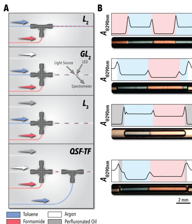
**Figure 1.** Plug-and-play MF configurations. (A) Schematic of commercial fluidic junctions and fluoropolymer tubing configurations used to attain two- to four-phase segmented flow regimes. (B) Temporal absorption measurement at 290 nm for each of the sample flow regimes with corresponding representative images.
