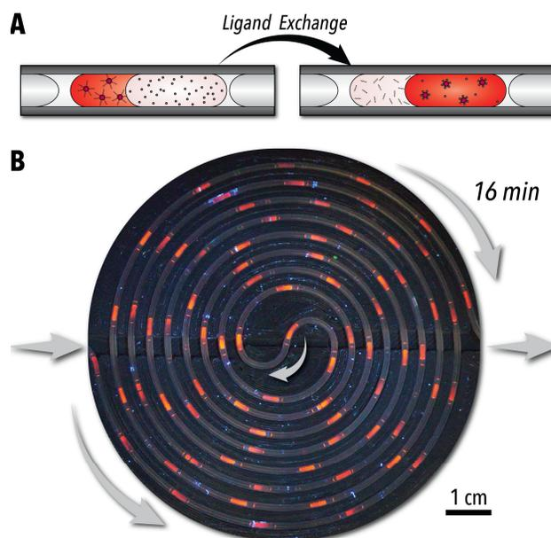
**Figure 4.** Biphasic ligand exchange of CdSe QDs in flow. (A) Schematic of the biphasic ligand exchange process where oleic acid-capped CdSe QDs transition from toluene to formamide to produce sulfide ligand-capped CdSe QDs. (B) Image of the continuous biphasic ligand exchange reaction in flow within the adjustable length spiral microreactor under UV illumination.
