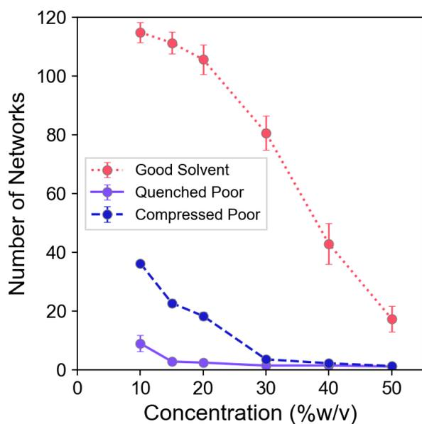
Fig. 5 Number of networks vs CPE concentration. Each point is averaged over 50  $\kappa\tau$ . Error bars represent one standard deviation. The threshold electronic coupling value for two monomers being connected is 0.02 eV
