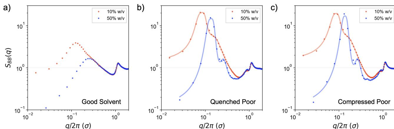
Fig. 3 Partial structure factor of the CPE backbone beads in (a) good solvent, (b) poor solvent quenched, and (c) poor solvent compressed at concentrations of 10% (red) and 50% (blue) w/v. The poor solvent data was fit to Equation 12. Values of  $q$  are divided by  $2\pi$  to aid interpretation, and  $1 \sigma \sim 0.5 \text{ nm}$  in real space.
