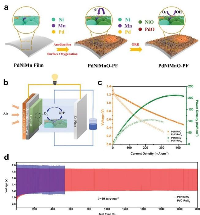
**Fig. 10** (a) Schematic illustration depicting the process of surface oxygenation of the PdNiMnO PFs catalyst. (b) The schematic illustration depicts the operating principle of an aqueous zinc-air flow
