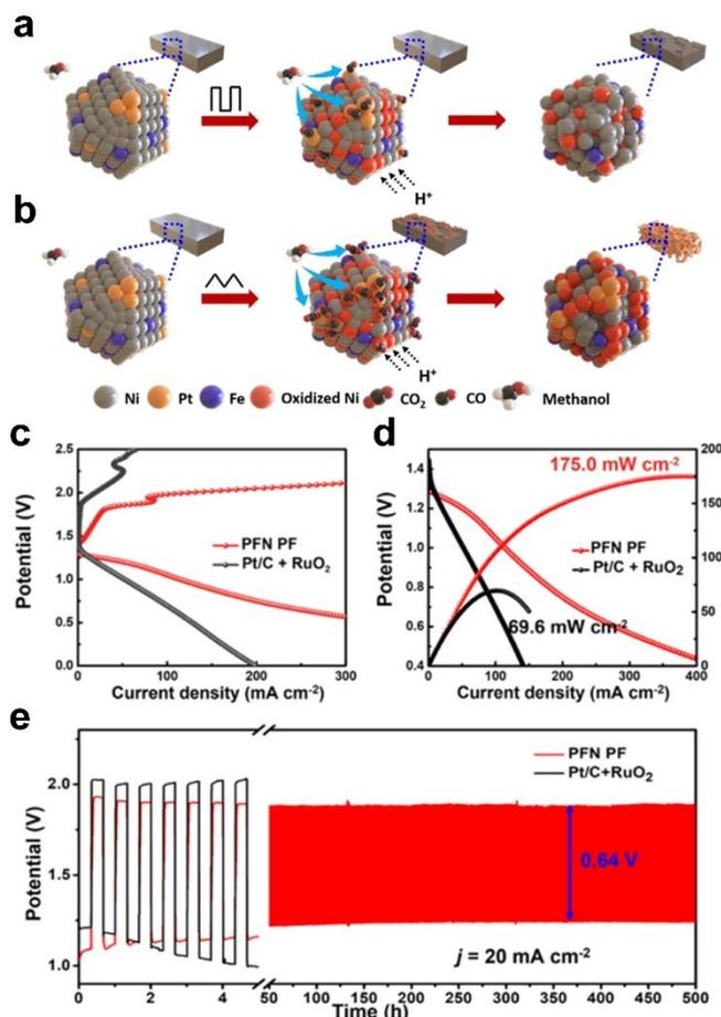
**Fig. 7** A schematic illustration of DCBT-directed synthesis utilizing (a) square-wave voltage and (b) triangular-wave voltage. (c) charge/discharge polarization curves, (d) power density curves, and (e) stability for ZABs with Pt<sub>1.1%</sub>Fe<sub>8.8%</sub>Ni PF and Pt/C+RuO<sub>2</sub> as air-electrode at a current density of 20 mA cm<sup>-2</sup>. Adapted with permission from ref. <sup>43</sup> Copyright 2021, ACS Publications.
