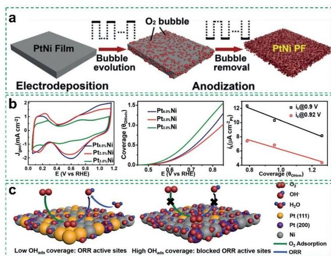
**Fig. 6** (a) An illustration of the process for fabricating PtNi PFs using DOBT. (b) The CV curves, reversible OH<sub>ads</sub> coverage, and the specific kinetic current densities of different samples at different potentials. (c) The illustration depicts the ORR process on low and high OH<sub>ads</sub> coverage. Adapted with permission from ref. <sup>99</sup> Copyright 2019, Wiley-VCH GmbH.
