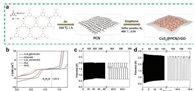
**Fig. 14** (a) A diagram illustrating the production process for the CoS<sub>x</sub>@PCN/rGO. (b) The bifunctional ORR/OER performance of different samples. Cycling curves for rechargeable ZABs at a current of 50 mA for (c) CoS<sub>x</sub>@PCN/rGO and (d) Pt/C+RuO<sub>2</sub>. Adapted with permission from ref.<sup>96</sup> Copyright 2018, Wiley-VCH GmbH.
