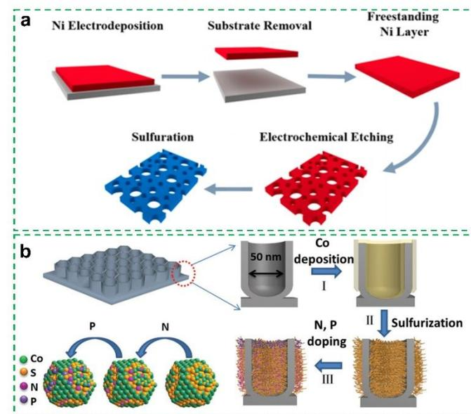
**Fig. 13** (a) A diagram illustrating the production process for the  $\text{NiS}_x$  FHF. Adapted with permission from ref. <sup>95</sup> Copyright 2018, ACS Publication. (b) A fabrication process of the N,P/CoS $_2$ @TiO $_2$  NPFs. Adapted with permission from ref. <sup>94</sup> Copyright 2018, Wiley-VCH GmbH.
