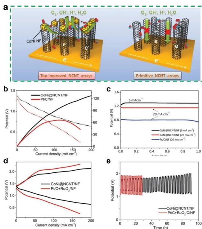
**Fig. 15** (a) Schematic illustrates the apically dominant mechanism of CoNi@NCNT/NF. (b) ZABs polarization curves and power density curves. (c) Discharge curves at 5 and 20 mA cm<sup>-2</sup>. (d) Discharge and charge polarization curves. (e) Cycling curves for rechargeable ZABs at a current of 5 mA cm<sup>-2</sup> for CoNi@NCNT/NF and Pt/C+RuO<sub>2</sub>/NF. Adapted with permission from ref.<sup>97</sup> Copyright 2018, Wiley-VCH GmbH.
