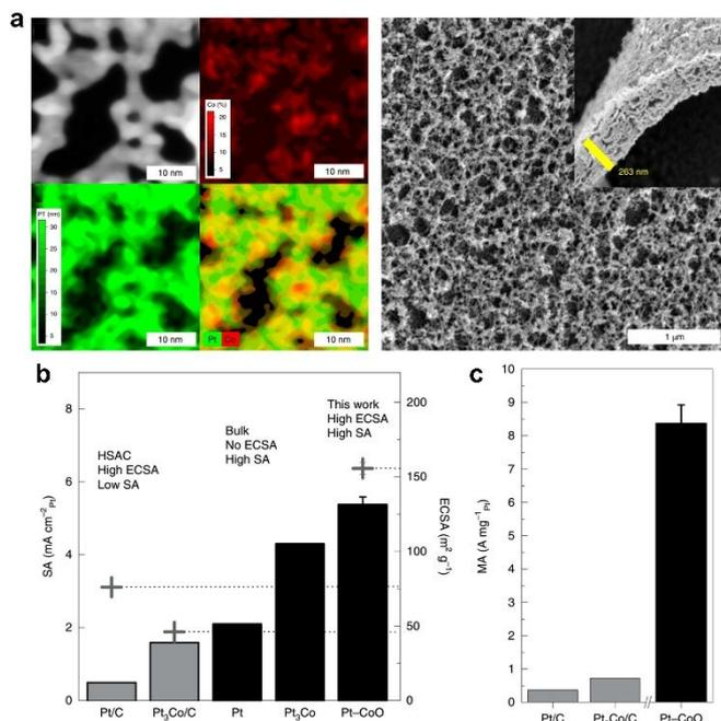
**Fig. 9** (a) High-angle annular dark-field (HAADF) scanning transmission electron microscopy (STEM) and scanning electron microscopy (SEM) images of self-supported nanoporous Pt-CoO networks. (b) ORR-specific activity (SA) and ECSA of Pt-CoO and other control samples. (c) ORR mass activity (MA) of Pt-CoO and other control samples. Adapted with permission from ref.<sup>73</sup> Copyright 2021, Springer Nature.
