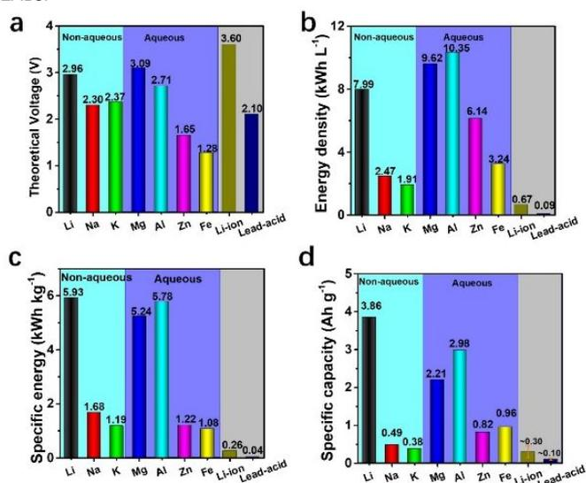
**Fig. 1.** (a) Theoretical voltage, (b) energy density, (c) specific energy, and (d) specific capacity between metal-air batteries, lead-acid batteries, and lithium-ion batteries. Reproduced with permission from ref. <sup>15</sup>. Copyright 2021 Wiley-VCH GmbH.
