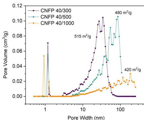
Figure 2. Pore size distributions of CNFPs determined by nitrogen physisorption using the DFT model.
