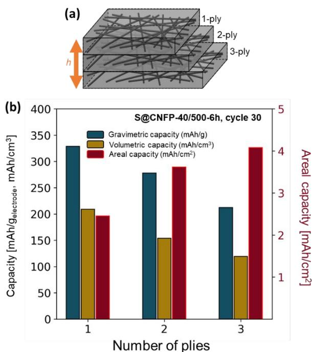
Figure 7. (a) Schematic of multi-ply CNFPs and (b) the gravimetric, volumetric, and areal capacities of these multi-ply papers.
