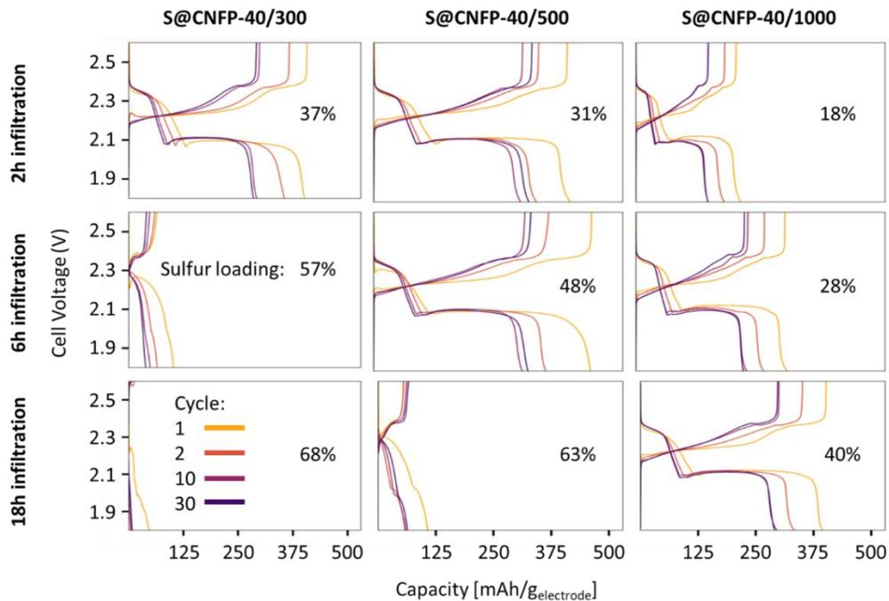
Figure 4. Charge–discharge curves of S@CNFPs with different sulfur infiltration durations.
