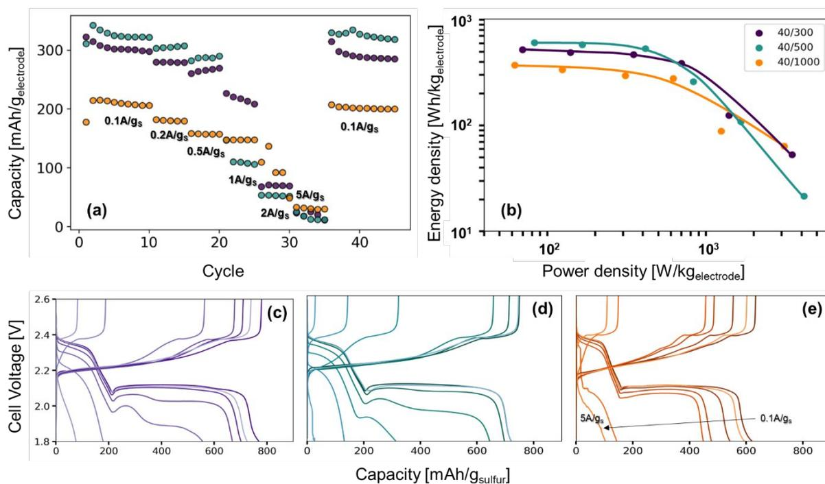
Figure 6. (a) Rate study of Li–S coin cells from 0.1A/g<sub>sulfur</sub> to 5A/g<sub>sulfur</sub>, (b) the Ragone plot produced from the third cycle of each rate, and (c–e) their corresponding charge–discharge curves.
