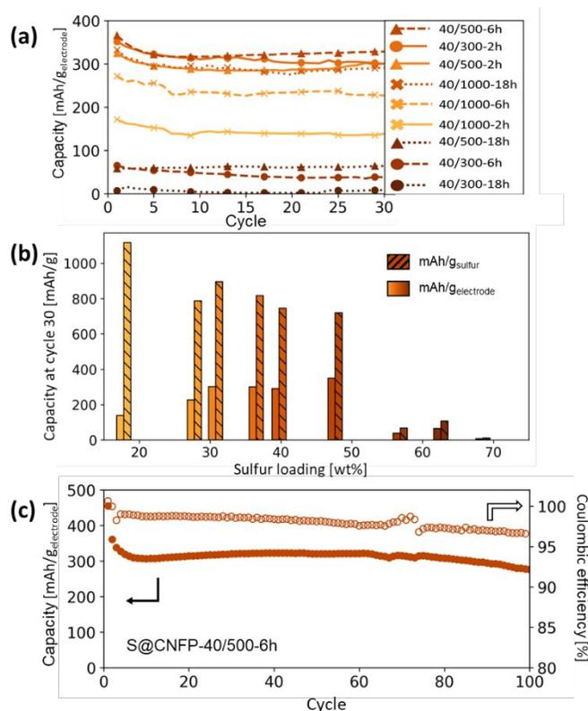
Figure 5. (a) Summary of Li-S cycling capacities at 0.1C for CNFPs using different sulfur infiltration durations and (b) their corresponding gravimetric capacities per weight sulfur and per total electrode weight after cycle 30 versus their sulfur weight loadings. (c) Long-term cycling of the S@CNFP-40/500-6h sample to 100 cycles. Results are summarized in Table S4, and cycling capacity normalized to sulfur mass is shown in Figure S5.
