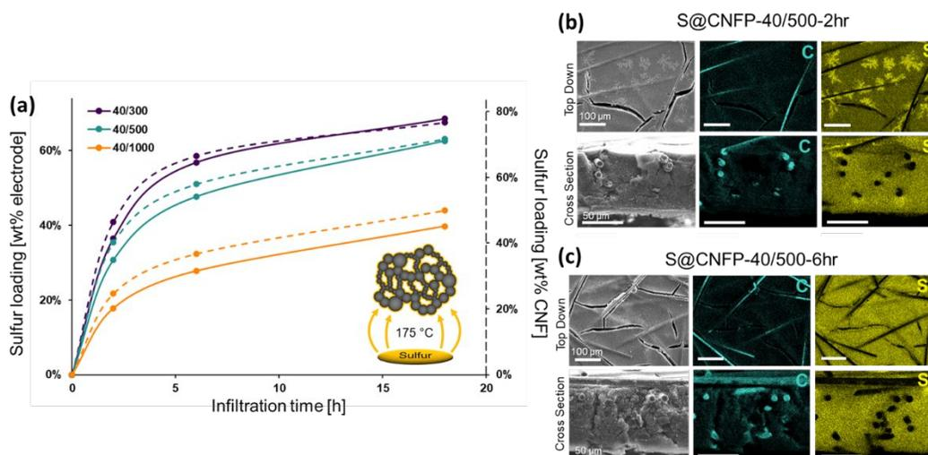
Figure 3. (a) Mass uptake by CNFPs upon vapor infiltration of  $S_8$  as a function of time: solid line represents the measured mass uptake in the CNFP, and the dotted line shows the mass of  $S_8$  uptake relative to the carbon nanofoam component of the CNFP. Scanning electron microscopy and cross-sectional EDS analysis of C and S for (b) 2 h and (c) 6 h infiltrations.
