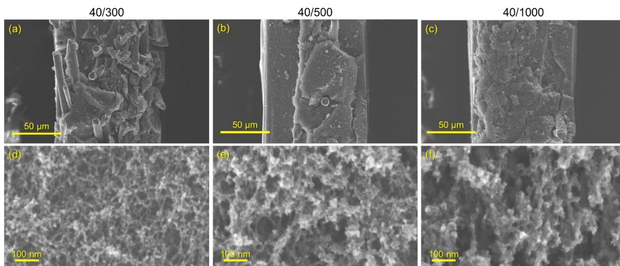
Figure 1. Scanning electron micrographs of 1-ply CNFP cross-sections for CNFP-40/300 (a), CNFP-40/500 (b), and CNFP-40/1000 (c), and their respective magnified images (d-f). In (a-c), the carbon nanofoam appears as a solid filling the gaps in the carbon fiber paper, and the pores are only visible at much higher magnifications (d-f).
