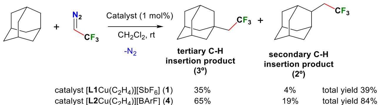
**Scheme 1.** Functionalization of C(sp<sup>3</sup>)-H bonds via carbene insertion mediated by **1** and **4**
