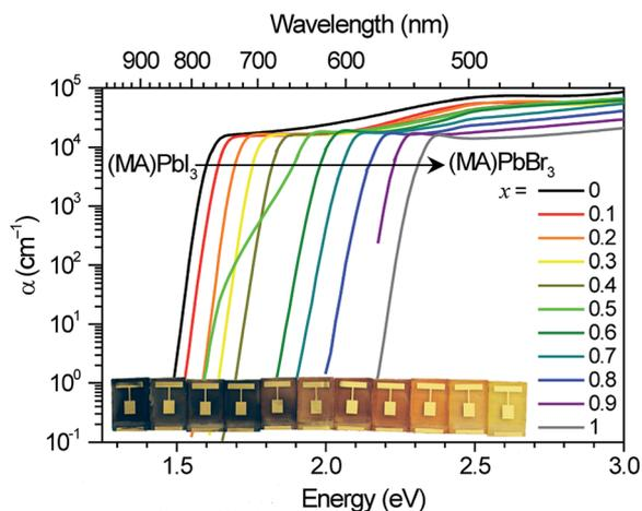
Fig. 1 Absorption coefficient of  $(\text{MA})\text{Pb}(\text{Br}_x\text{I}_{1-x})_3$  measured by diffuse spectral reflection and transmission measurements on thin films and photocurrent spectroscopy of solar cells. Inset: photograph of  $(\text{MA})\text{Pb}(\text{Br}_x\text{I}_{1-x})_3$  photovoltaic devices from  $x = 0$  to  $x = 1$  (left to right).
