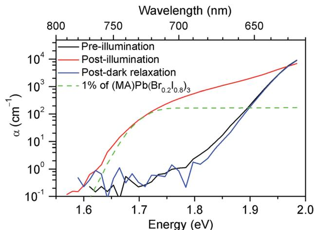
Fig. 3 Absorption spectra of an  $x = 0.6$  film before (black) and after (red) white-light soaking for 5 minutes at  $100 \text{ mW cm}^{-2}$ , and after 1 h in the dark (blue). A scaled absorption spectrum of an  $x = 0.2$  film (dashed green) is shown for comparison.
