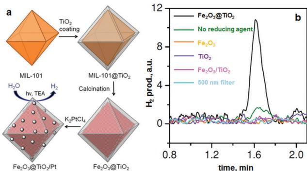
Fig. 4 (a) MOF-templated synthesis of  $\text{Fe}_2\text{O}_3@TiO_2$  by coating MIL-101(Fe) with  $TiO_2$  followed by calcination, and its use for photocatalytic hydrogen production after depositing Pt particles; (b) the  $H_2$  peaks in GC analysis of the headspace using 0.5 mg of different catalyst samples. From de Krafft *et al.* 2012.<sup>110</sup> Copyright © 2012 by John Wiley Sons, Inc. Reprinted by permission of John Wiley & Sons, Inc.
