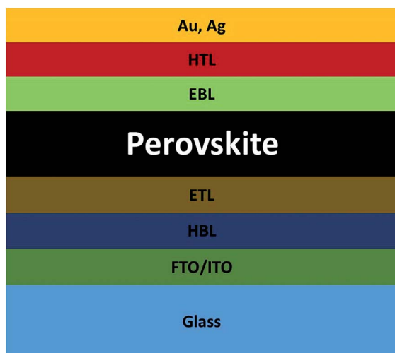
Fig. 1 Schematic of perovskite solar cell.
