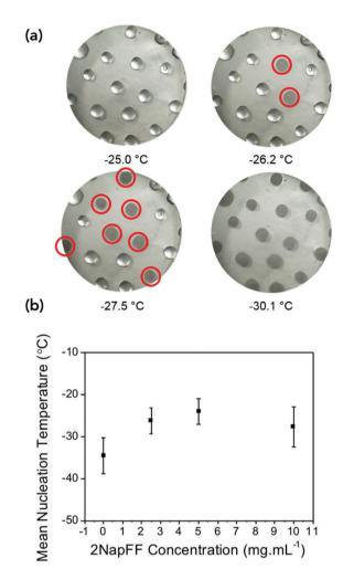
Fig. 3 Ice nucleation assay. (a) Example multi-point freezing assay used to assess the nucleation temperature as the temperature is reduced. Nucleating droplets are circled in red. (b) Mean nucleation temperature as a function of gelator concentration.
