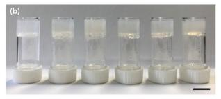
Fig. 1 (a) Chemical structure of gelator 2NapFF. (b) Photographs of 2NapFF at (left to right) 10 mg  $mL^{-1}$ , 5 mg  $mL^{-1}$ , 2.5 mg  $mL^{-1}$ , 20 : 80 glycerol : water (5 mg mL $^{-1}$ ), 40:60 glycerol: water (5 mg mL $^{-1}$ ) and 60:40 glycerol: water  $(5 \text{ mg mL}^{-1})$ . Scale bar is 1 cm.
