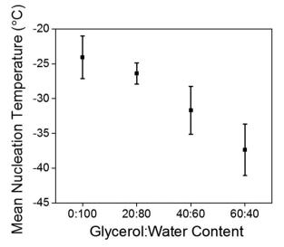
Fig. 5 Mean nucleation temperature of LMWG formed in presence of glycerol.
