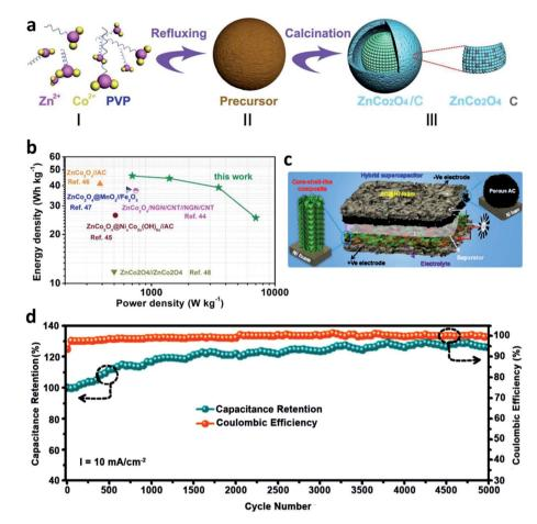
Fig. 4 (a) Scheme of the synthesis a yolk-shell structure  $ZnCo_2O_4$  material, (b) Ragone plots of AACSDs (modified from ref. 85, copyright permission from the Royal Society of Chemistry); (c) illustration for the preparation process and (d) cycling stability of core-shell-like NiO@Co<sub>3</sub>O<sub>4</sub>-NiO FTN/Ni foam (modified from ref. 88, copyright permission from Elsevier).
