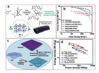
**Fig. 7** (a) Schematic of N-NbOC material, (b) Ragone plot of N-NbOC//AC (modified from ref. 116, copyright permission from Elsevier); (c) schematic of the process for fabricating the TNO/HG electrode, (d) Ragone plot of TNO/HG//AC with other LIHSCDs (modified from ref. 118, copyright permission from Elsevier).
