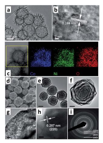
Fig. 1 (a–c) TEM images and EDS mapping of three dimensional NiCo<sub>2</sub>O<sub>4</sub> nanospheres, (d–i) SEM and TEM images of seven-layered Ni–Co oxide spheres derived from MOF (modified from ref. 32 and 33, copyright permission from Elsevier and Wiley-VCH, respectively).
