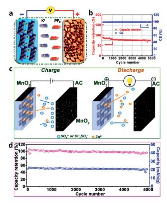
Fig. 9 (a) Schematic and (b) long-term cycling stability at the current density of 1 A  $g^{-1}$  of a NGC//KTO KIHSCD (modified from ref. 125, copyright permission from the American Chemical Society); (c) schematic illustration and (d) cycling stability of a designed MnO<sub>2</sub>//AC ZIHSCD (modified from ref. 126, copyright permission from Elsevier).
