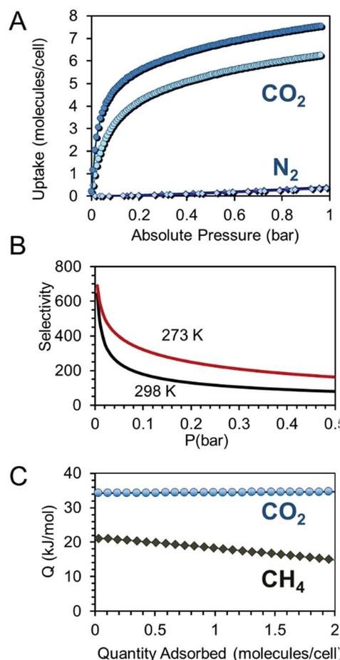
Fig. 2 (A) CO<sub>2</sub> and N<sub>2</sub> isotherms of CPOS-5 collected at 273 K (blue circles and diamonds, respectively) and 298 K (light-blue circles and diamonds, respectively). (B) CO<sub>2</sub>/N<sub>2</sub> selectivity values of CPOS-5 versus pressure calculated starting from a 15/85 mixture and applying IAST calculation. (C) Isothermic heats of adsorption (*Q*<sub>st</sub>) versus CO<sub>2</sub> and CH<sub>4</sub> loading.
