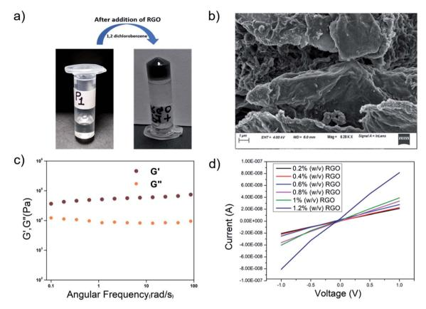
Fig. 10 (a) The reduced graphene oxide incorporated hybrid organogel RGO-P1. (b) An FESEM image of the RGO-P1 hybrid organogel. (c) Frequency dependence of the dynamic storage modulus (G') and the loss modulus (G') of the RGO-P1 hybrid organogel (1 wt%) in 1,2-DCB. (d) I-V curve showing the conductivity of the hybrid organogels upon RGO incorporation.
