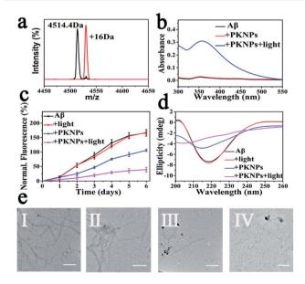
Fig. 3 (a) The mass spectra of  $A\beta_{42}$  and  $A\beta_{42}$  oxidized by PKNPs under laser excitation. (b) DNPH assay. (c) ThT fluorescence assay. (d) CD spectra of A $\beta$  after various treatments. (e) TEM images of different A $\beta$  samples: (l) A $\beta$ , (II) A $\beta$  + light, (III) A $\beta$  + PKNPs, and (IV) A $\beta$  + PKNPs + light. Scale bars are 200 nm.
