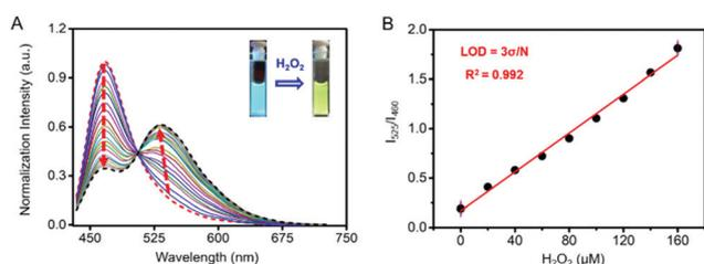
**Fig. 2** Sensitivity and selectivity of **Cm-Np-B@BSA** (5/50  $\mu\text{M}$ ) for  $\text{H}_2\text{O}_2$  detection. (A) Fluorescence spectral response of **Cm-Np-B@BSA** (5/50  $\mu\text{M}$ ) to  $\text{H}_2\text{O}_2$  at the concentration of 0–200  $\mu\text{M}$ ; (B) linear detection range and limit of detection (LOD) of **Cm-Np-B@BSA** (5/50  $\mu\text{M}$ ). All measurements were carried out in PBS buffer, pH 7.4, excitation wavelength: 410 nm.
