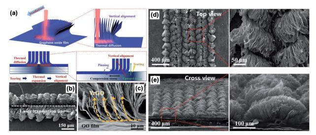
**Fig. 11** Vertical alignment of reduced graphene oxide nanosheets by laser irradiation. (a) Schematic of the CO<sub>2</sub> laser irradiation fabrication process of the vertically aligned nanostructure. (b and d) Top view of the vertically aligned nanosheets. (c and e) Cross-sectional view of the as-fabricated nanostructure. Reproduced from ref. 186 with permission from Elsevier.
