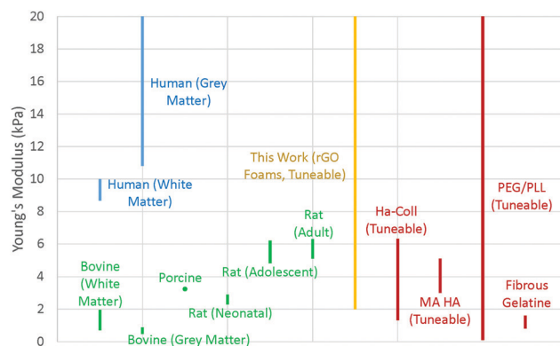
Fig. 2 Mechanical properties for brain tissues of different species, and of other tissue scaffolds designed for brain cell research, as reported in literature (Table S2, ESI†). Where the modulus was not explicitly provided, these values were calculated by computing the ratio of stress to strain in the linear region of the data values as quoted in the literature.
