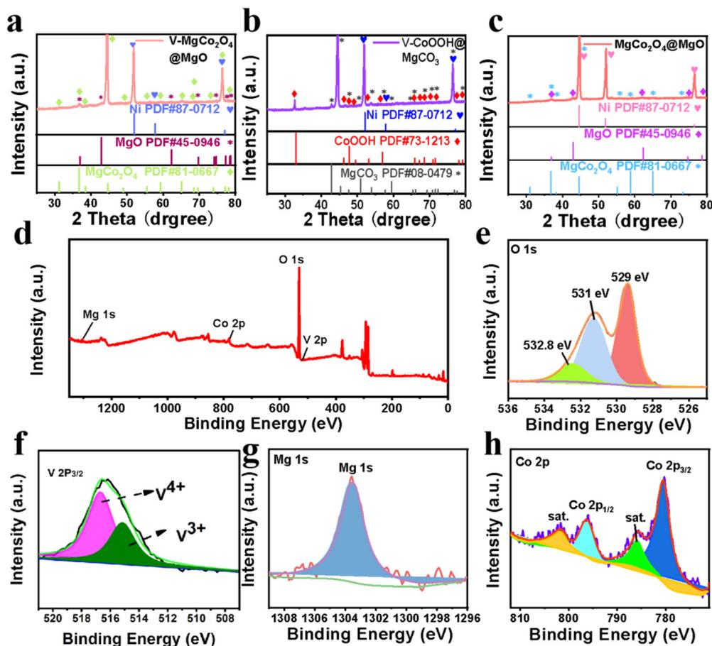
Fig. 2 XRD and XPS analyses. XRD spectra of (a) V-MgCo<sub>2</sub>O<sub>4</sub>@MgO, (b) V-CoOOH@MgCO<sub>3</sub> and (c) MgCo<sub>2</sub>O<sub>4</sub>@MgO. (d) XPS survey spectrum of V-MgCo<sub>2</sub>O<sub>4</sub>@MgO. XPS spectra of (e) O 1s, (f) V 2p, (g) Mg 1s, and (h) Co 2p for V-MgCo<sub>2</sub>O<sub>4</sub>@MgO.
