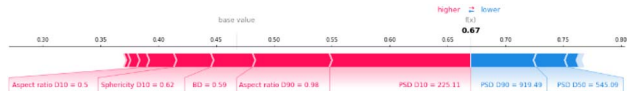
Fig. 16 SHAP force plot of the prediction of the cohesive material from the external validation that was classified as free-flowing by step 1. The red bars of the plot show the drivers that are pushing the classification toward free-flowing and the blue bars show the drivers that are pushing the classification towards non-free flowing.
