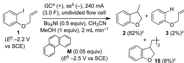
**Scheme 4** Selective electroreductive cyclisation of aryl iodide **1** in an undivided electrochemical flow cell, using a highly reducing catalytic mediator. <sup>a</sup> Glassy carbon anode. <sup>b</sup> Stainless steel cathode. <sup>c</sup> Yields are estimated using calibrated GC.
