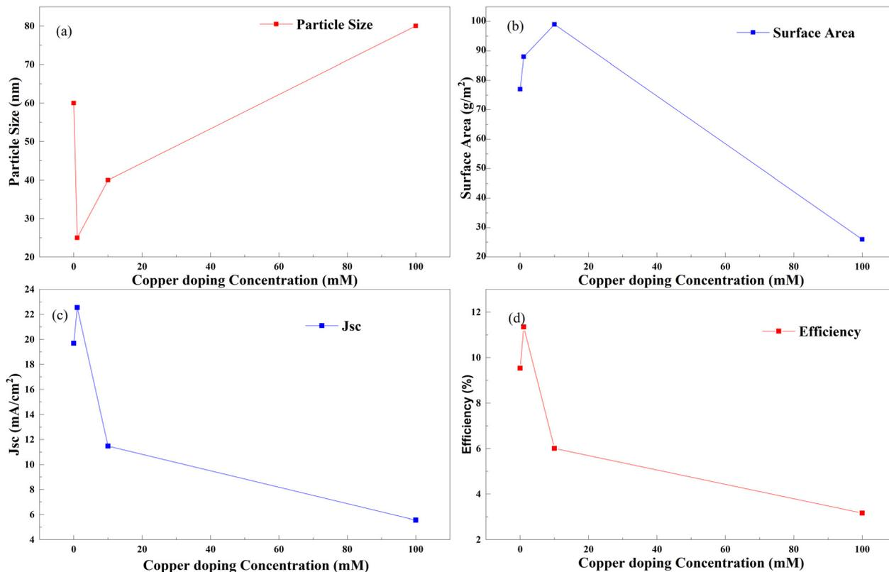
Fig. 33 Copper doping concentration with (a) particle size, (b) surface area, (c)  $J_{sc}$  and (d) efficiency.<sup>137</sup>
