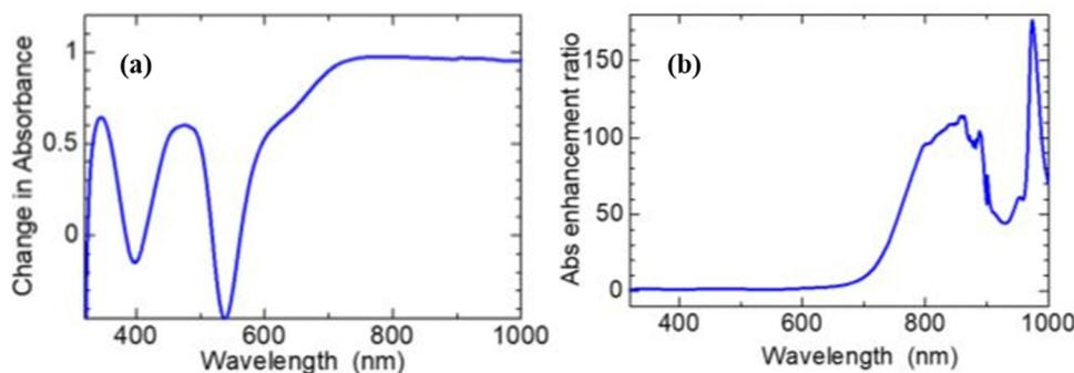
Fig. 20 Optical absorption spectra showing enhanced broadband light absorbance of the N719 dye: (a) absorbance of  $[0.12 \text{ mg mL}^{-1} \text{ dye}] - \text{absorbance of [dye-only]}$ . (b) The absorbance of  $[0.12 \text{ mg mL}^{-1} \text{ dye}] - \text{absorbance of [dye-only]}$ .<sup>176</sup>
