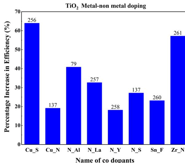
Fig. 31 Increase in PCE with metal-nonmetal codoped TiO<sub>2</sub>. Data points are labelled with references.
