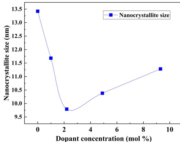
Fig. 15 Influence of Nb doping on the average size of  $\text{TiO}_2$  nanoparticles.<sup>173</sup>
