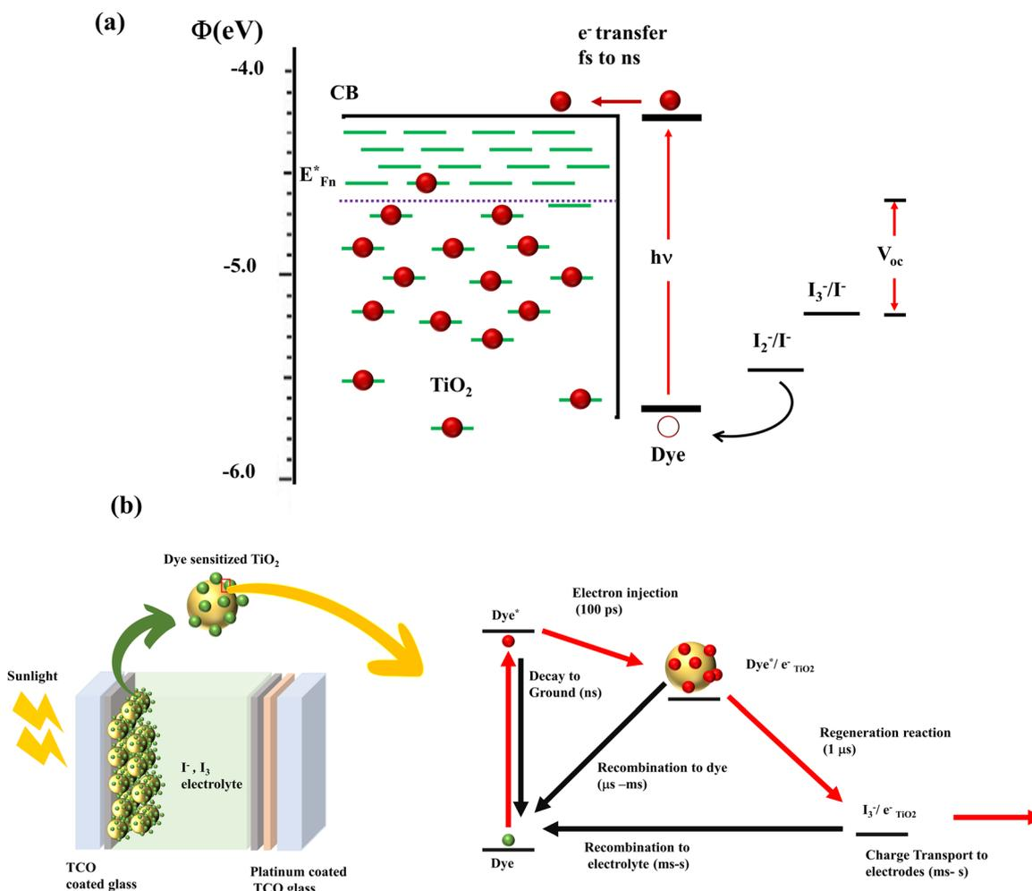
Fig. 3 (a) Illustration of the energy level of the DSSC.<sup>20</sup> (b) Charge transfer and recombination mechanisms involved in the DSSC.<sup>27</sup>
