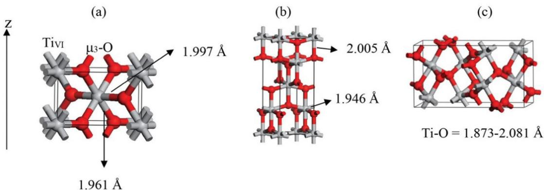
Fig. 2 Structures of  $\text{TiO}_2$  natural polymorphs: (a) rutile, (b) anatase and (c) brookite.<sup>17</sup>
