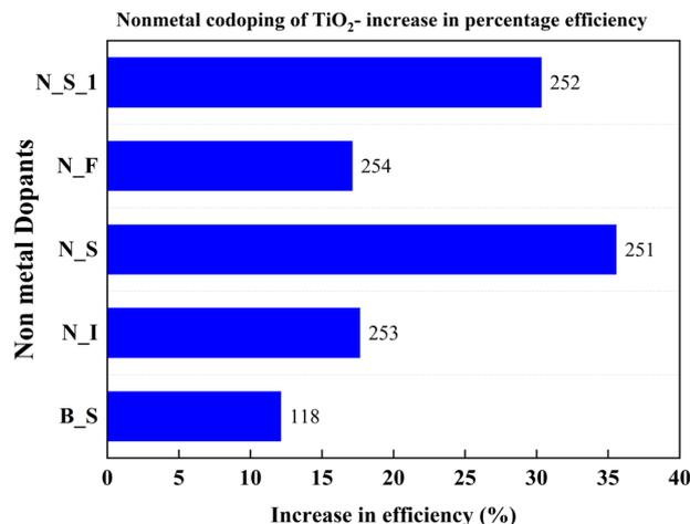
Fig. 30 Increase in PCE of nonmetal codoped TiO<sub>2</sub>. Data points are labelled with references.
