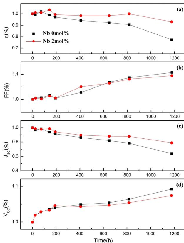
Fig. 16 Variation of  $V_{oc}$ ,  $J_{sc}$ , FF and efficiency with time for Nb doped DSSCs. Reproduced from ref. 142 with permission from Elsevier.<sup>142</sup>
