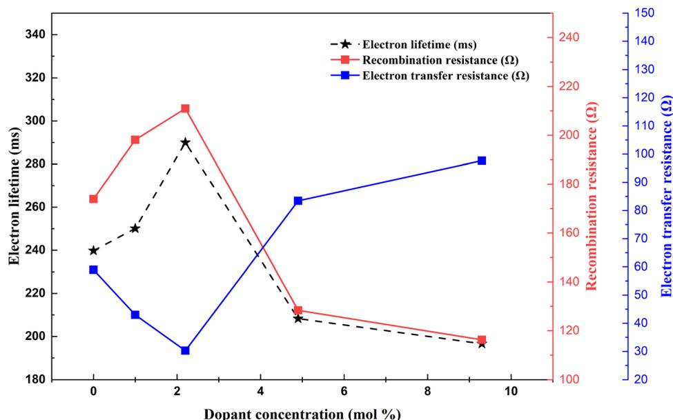
Fig. 18 Nd dopant electron lifetime, recombination resistance and electron transfer resistance correlation.<sup>138</sup>
