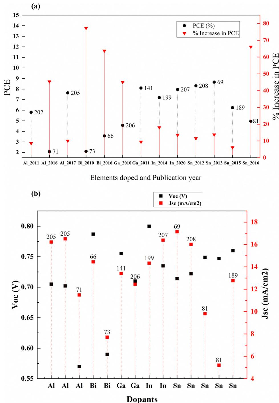
Fig. 23 (a) Percentage increase in PCE in post-transition metals with doping. (b)  $J_{sc}$  and  $V_{oc}$  of post-transition metals when doped into  $TiO_2$  for DSSC fabrication. Data points are labelled with references.
