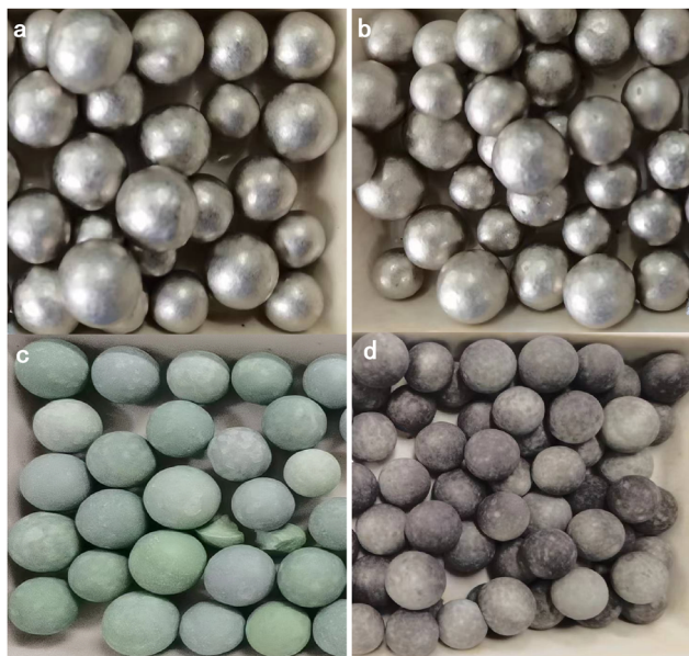
Fig. 2 Appearance of (a) fresh and (b) used Ir/Ni. Appearance of (c) fresh and (d) used Ir-Ni/Al 2 O 3 catalysts.
