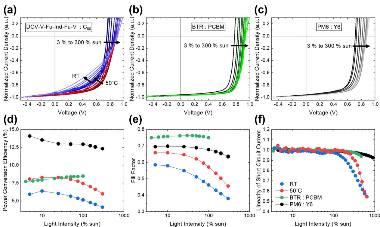
**Fig. 2** (a)–(c) Normalised *JV*-curves of DCV-V-Fu-Ind-Fu-V : C<sub>60</sub> (RT and 50 °C, blue and red, respectively), BTR:PCBM and PM6:Y6, respectively, for the range of 3% to 300% of 1 sun equivalent light intensity. (d)–(f) Light intensity dependence of power conversion efficiency, fill factor and linearity of the short circuit current density, respectively. See (f) for the legend.
