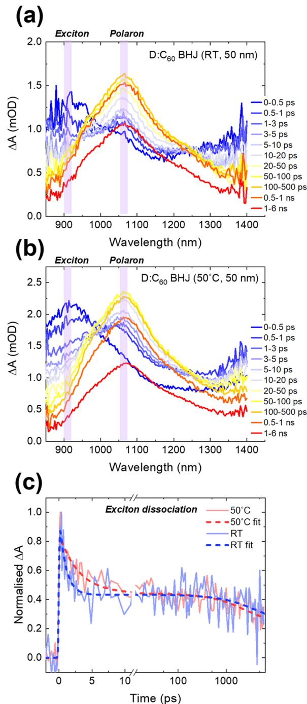
Fig. 5 (a) and (b) Transient absorption spectra of RT and 50 °C films, respectively, after selectively pumping the donor at 600 nm with a fluence of  $6 \mu\text{J cm}^{-2}$ . (c) Time evolution of the exciton decay signal with lifetimes of 0.9 and 2.9 ps for RT and 50 °C, respectively.
