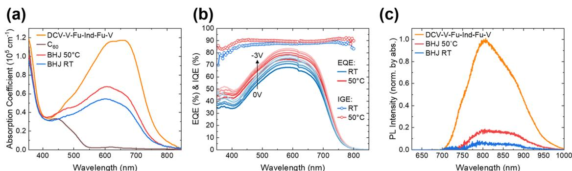
Fig. 4 (a) Absorption spectra of the neat donor DCV-V-Fu-Ind-Fu-V, acceptor C<sub>60</sub> and blend films deposited at 50 °C and room temperature. (b) Field-dependent external quantum efficiency (EQE) spectra of the 50 °C and RT devices. Also shown is the internal generation efficiency (IGE) that was calculated as the ratio of the EQE at 0 V and -3 V. (c) Donor photoluminescence spectra of the neat donor, RT and 50 °C blends normalized by their absorption.
