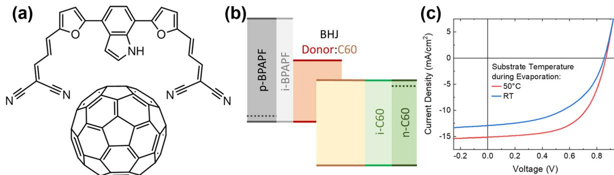
**Fig. 1** (a) Chemical structure of the donor molecule DCV-V-Fu-Ind-Fu-V and the acceptor C<sub>60</sub>. (b) Schematic of the relative energy levels of the active layer and interlayers. Note that the relative energetic alignment is deduced from a combination of literature and experimental values as described in the main text. (c) *JV*-curve of the devices with 50 nm active layer thickness used for the analysis herein.
