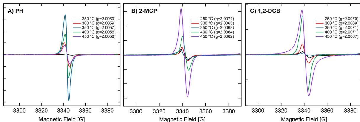
**Fig. 3** Representative ESR spectra for the formation of EPFRs for three organic precursors on ZnO NPs. (A) The ESR spectra of ZnO NPs (20 nm) and 2-MCP at 250, 300, 350, 400, and 450 °C at 14 Torr. (B) The ESR spectra of ZnO NPs (20 nm) and PH at 250, 300, 350, 400, and 450 °C at 14 Torr. (C) The ESR spectra of ZnO NPs (20 nm) and 1,2-DCB at 250, 300, 350, 400, and 450 °C at 14 Torr.
