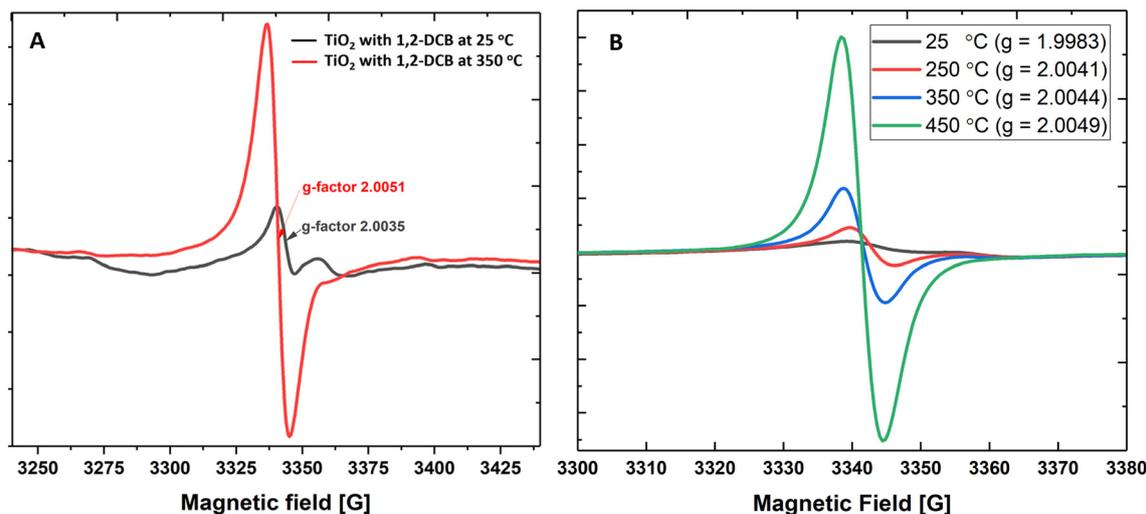
Fig. 1 (A) The ESR intensity of  $\text{TiO}_2$  NPs and 1,2-DCB at low temperature (25 °C) and at high temperature (350 °C) at 670 Torr. (B) The ESR intensity of  $\text{TiO}_2$  NPs and 2-MCP at 25, 250, 350, and 450 °C at 670 Torr.
