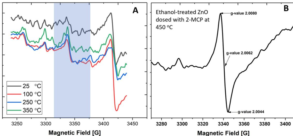
**Fig. 2** (A) The ESR spectra of ZnO NPs (30 nm) and 2-MCP at 25, 100, 250, and 350 °C at 670 Torr. The shaded region is the magnetic field window for organic radicals (EPFRs). (B) The ESR spectra of ZnO NPs and 2-MCP at 450 °C, pretreated with ethanol at 670 Torr.
