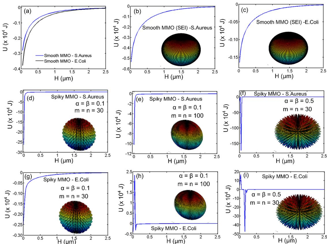
Fig. 8 DLVO interaction energy between MMO and bacteria (*S. aureus* and *E. coli*) using (a) DA approximation and (b)–(i) SEI technique. (a)–(c) are for smooth spheres and (d)–(i) are obtained for spiky MMO with different densities of spikes ( $m$ ,  $n$ ) and spike aspect ratios ( $\alpha$ ,  $\beta$ ).
