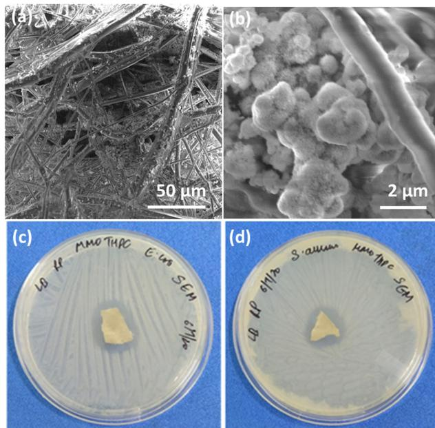
Fig. 10 FESEM images of MMO-Ag coated on the meltblown fabric (a) low magnification and (b) high magnification. Photographs of the MMO-Ag-coated meltblown fabric showing the ZI against (c) *E. coli* and (d) *S. aureus*.
