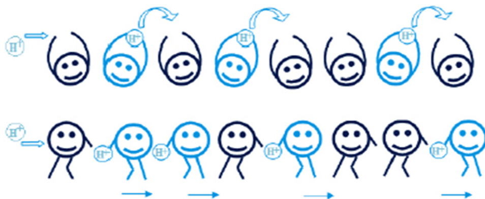
Fig. 4 A schematic representation of the Grotthuss and vehicular mechanisms. 31
