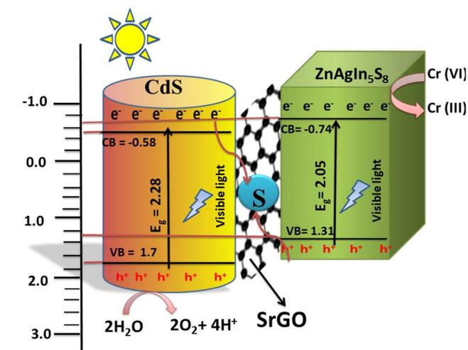
Scheme 2 Photocatalytic mechanism of Cr(vi) reduction using Zn-AgIn<sub>5</sub>S<sub>8</sub>/S-rGO/CdS nanocomposite.
