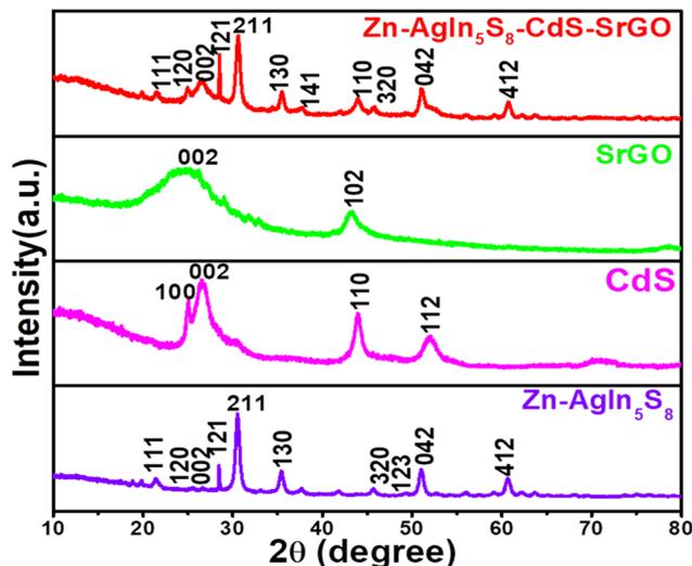
Fig. 1 XRD patterns of the prepared Zn-AgIn<sub>5</sub>S<sub>8</sub>, CdS, SrGO, Zn-AgIn<sub>5</sub>S<sub>8</sub>/CdS/SrGO NMs.
