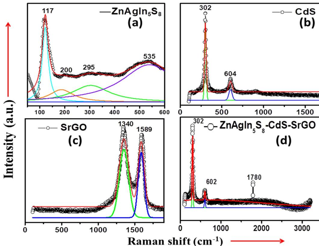
Fig. 4 Raman shift vs. Intensity of (a) Zn-AgIn<sub>5</sub>S<sub>8</sub>, (b) CdS, (c) SrGO, and (d) Zn-AgIn<sub>5</sub>S<sub>8</sub>/CdS/SrGO nanocomposite.
