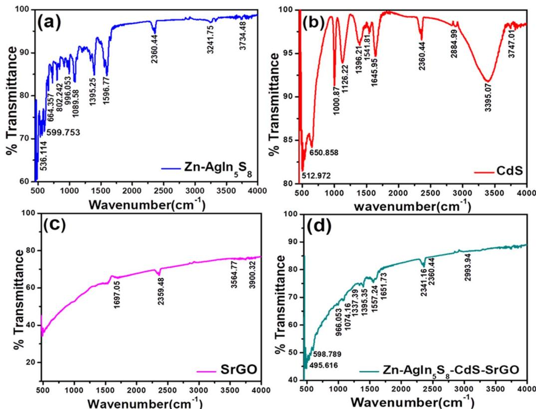
Fig. 2 FTIR study of (a) of Zn-AgIn<sub>5</sub>S<sub>8</sub> (b) CdS (c) SrGO and (d) Zn-AgIn<sub>5</sub>S<sub>8</sub>/CdS/SrGO nanocomposite.
