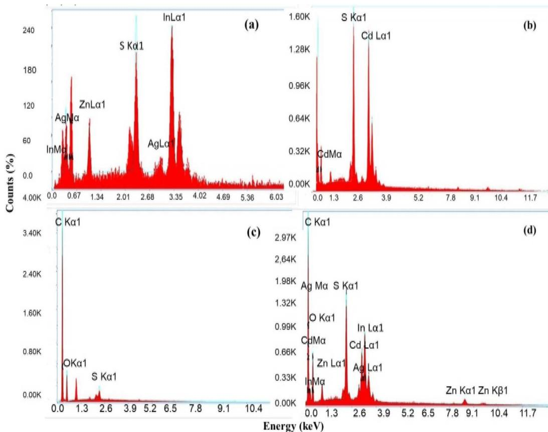
Fig. 6 EDX spectra of the synthesized nanomaterials (a) Zn-AgIn<sub>5</sub>S<sub>8</sub>, (b) CdS, (c) SrGO, and (d) Zn-AgIn<sub>5</sub>S<sub>8</sub>/CdS/SrGO.
