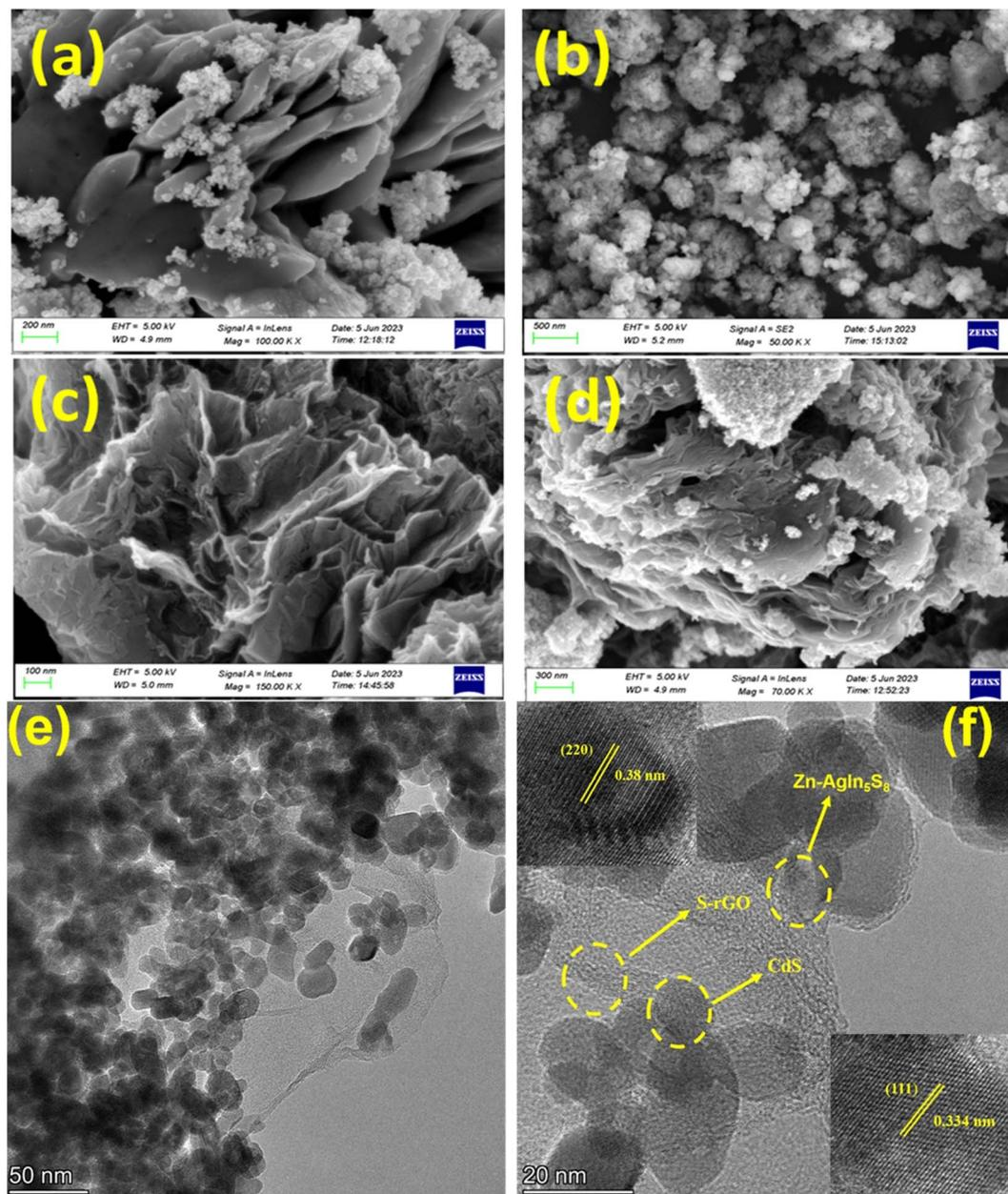
Fig. 5 FE-SEM micrographs of (a) Zn-AgIn<sub>5</sub>S<sub>8</sub>, (b) CdS, (c) SrGO, and (d) Zn-AgIn<sub>5</sub>S<sub>8</sub>/CdS/SrGO. (e) TEM image of Zn-AgIn<sub>5</sub>S<sub>8</sub>-CdS-S-rGO heterojunction, (f) HRTEM image of Zn-AgIn<sub>5</sub>S<sub>8</sub>-CdS-S-rGO heterojunction (inset: lattice fringes of Zn-AgIn<sub>5</sub>S<sub>8</sub> and CdS).
