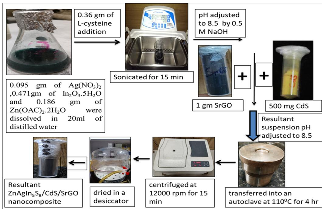
Scheme 1 Schematic illustration of the synthesis of Zn-AgIn<sub>5</sub>S<sub>8</sub>/CdS/SrGO nanocomposite.
