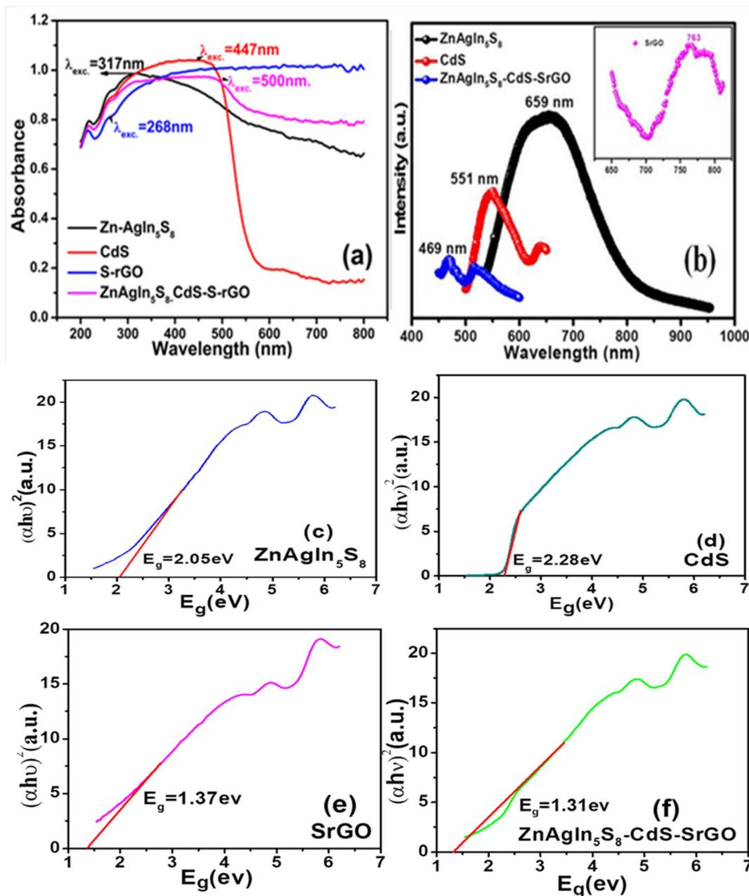
Fig. 3 (a) UV DRS study of Zn-AgIn<sub>5</sub>S<sub>8</sub>, CdS, Zn-AgIn<sub>5</sub>S<sub>8</sub>/CdS/SrGO NMs (b) PL spectra of Zn-AgIn<sub>5</sub>S<sub>8</sub>, CdS, SrGO, and Zn-AgIn<sub>5</sub>S<sub>8</sub>/CdS/SrGO nanocomposite. Tauc plot for calculating Bandgap energy of the synthesized NMs (c) Zn-AgIn<sub>5</sub>S<sub>8</sub> (d) CdS (e) SrGO (f) Zn-AgIn<sub>5</sub>S<sub>8</sub>/CdS/SrGO nanocomposite.
