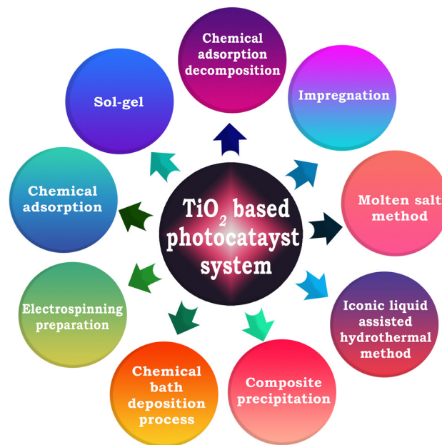
Fig. 16 Schematic representation of the various strategies for the synthesis of TiO 2 -based photocatalyst systems reported in the literature.
