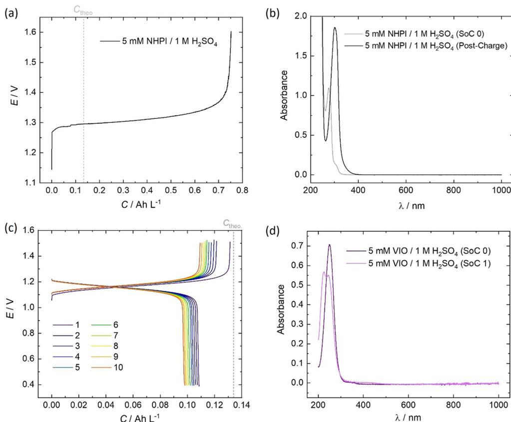
Fig. 7 RFC test of 5 mM organic in 100 mL electrolyte cycled galvanostatically at  $5 \text{ mA cm}^{-2}$  and *in-operando* recorded UV-vis spectra at key points during the initial cycle of (a) and (b) NHPI and (c) and (d) VIO.
