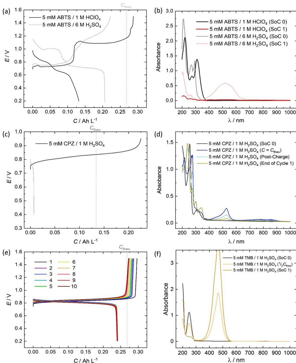
Fig. 6 RFC test of 5 mM organic in 100 mL electrolyte cycled galvanostatically at  $5 \text{ mA cm}^{-2}$  and *in-operando* recorded UV-vis spectra at key points during the initial cycle of (a) and (b) ABTS, (c) and (d) CPZ and (e) and (f) TMB.
