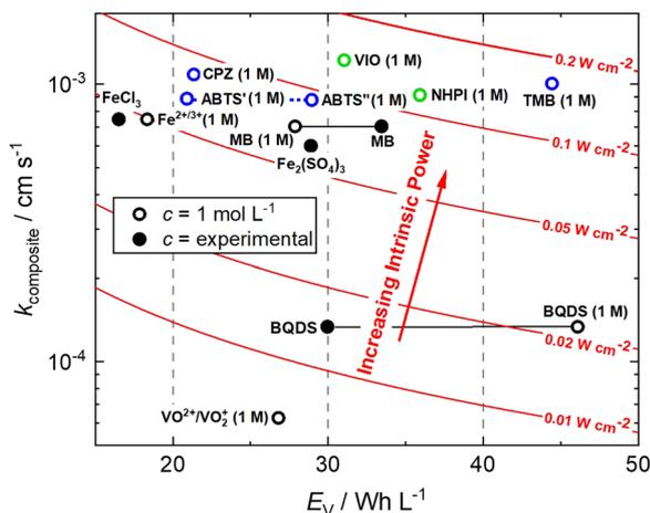
**Fig. 4** Intrinsic power of organic redox couples in a hypothetical  $\text{H}_2\text{-X}$  RFC.<sup>15,16,24,26–28</sup> ABTS: 2,2'-azinobis(3-ethylbenzothiazoline-6-sulfonate); BQDS: 2-dihydrobenzoquinone-3,5-disulfonic acid; CPZ: chlorpromazine; MB: methylene blue; NHPI: *N*-hydroxyphthalimide; TMB: *N,N,N',N'*-tetramethylbenzidine; VIO: violuric acid.
