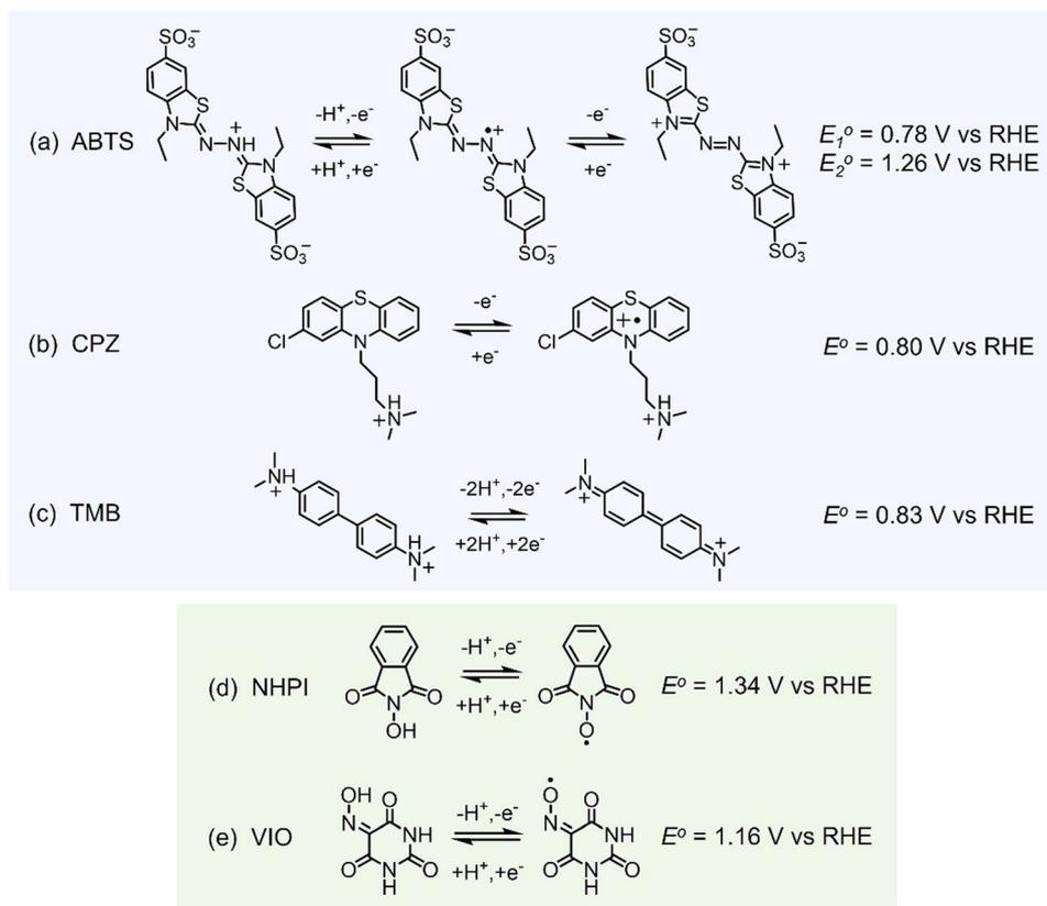
**Fig. 5** Determined redox reactions and potentials for (a) 2,2'-azinobis(3-ethylbenzothiazoline-6-sulfonate) (ABTS) in 1 M  $\text{HClO}_4$ , and (b) chlorpromazine (CPZ), (c) *N,N,N',N'*-tetramethylbenzidine (TMB), (d) *N*-hydroxyphthalimide (NHPI) and (e) violuric acid (VIO), in 1 M  $\text{H}_2\text{SO}_4$ .
