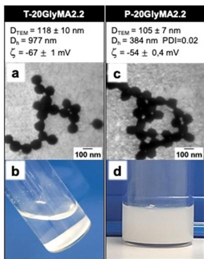
**Fig. 2** Surfactant-free latex prepared *via* SFEP of GlyMA at 60 °C (T-20GlyMA2.2) and under 405 nm irradiation at RT (P-20GlyMA2.2) using  $R = 20\%$  and SC = 2.2% w/w in water. (a and c) TEM images of latex immediately after synthesis. (b and d) Photographs of latex dispersions after three months in dark at RT.
