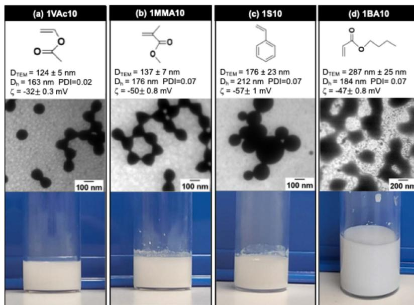
**Fig. 8** TEM images and photographs of surfactant-free latex dispersions prepared *via* photo-SFEP under 405 nm irradiation at  $R = 1\%$  and  $SC = 10\%$  w/w of various monomers: (a) vinyl acetate (VAc), (b) methyl methacrylate (MMA), (c) and styrene (S), and (d) *n*-butyl acrylate (BA).
