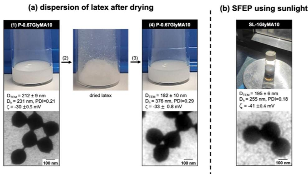
**Fig. 6** Sustainability of photo-SFEP process. (a) (1) Surfactant-free latex prepared via photo-SFEP of GlyMA under 405 nm irradiation using  $R = 0.67‰$  at SC = 10 w/w. (2) The nanoparticles were lyophilized and subsequently (3) re-dispersed in water targeting initial SC = 10 w/w. (b) Surfactant-free latex prepared via photo-SFEP of GlyMA under sunlight using  $R = 1‰$  at SC = 10 w/w in water.
