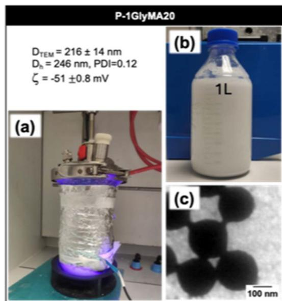
**Fig. 7** Scale-up of surfactant-free latex synthesis *via* photo-SFEP of GlyMA under 405 nm irradiation. (a) Reaction setup for the scale-up to 1 liter, using  $R = 1\%$  and  $SC = 20\%$  w/w. (b) The resulting stable latex dispersion produced in a 1 L batch. (c) TEM image of nanoparticles in the latex.
