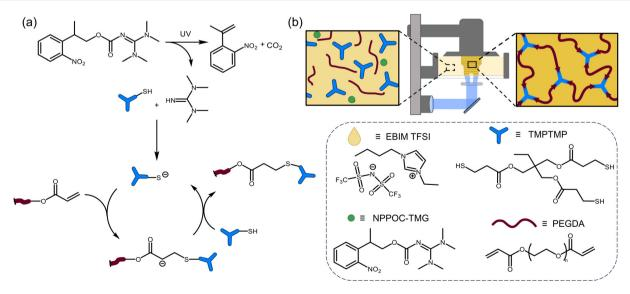
Fig. 1 Base-catalyzed thiol-Michael DLP printing (a) reaction mechanism for photolysis of PBG and thiol-Michael reaction, (b) cartoon of DLP printer and chemical structures of resin components.
