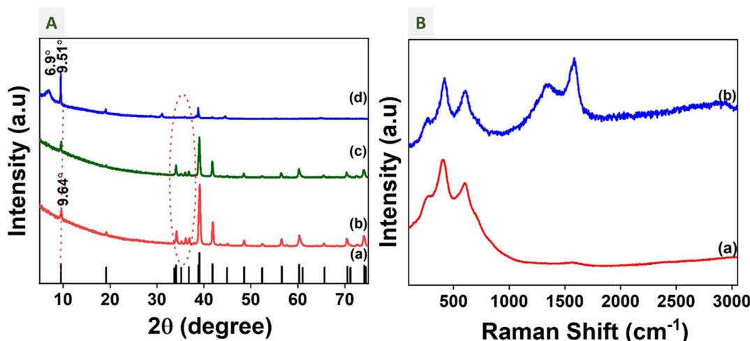
Fig. 2 Structural characterization: (A) XRD patterns of (a) ICDD 00-052-0875, (b)  $\text{Ti}_3\text{AlC}_2$ , (c) MSTC-00, and (d) MSTC-OX, and (B) Raman spectra of (a)  $\text{Ti}_3\text{AlC}_2$  and (b) MSTC-OX.
