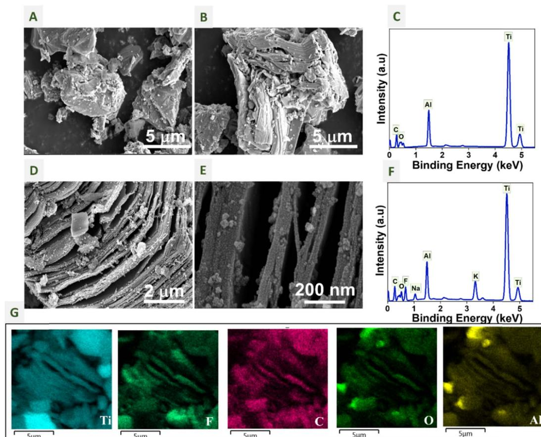
Fig. 3 Morphological and compositional characterization: SEM images of (A and B)  $\text{Ti}_3\text{AlC}_2$ , (D and E) MSTC-OX, energy dispersive X-ray spectra of (C)  $\text{Ti}_3\text{AlC}_2$  and (F) MSTC-OX and EDS mapping of MSTC-OX for the elements (G) Ti  $K\alpha$ , F  $K\alpha$ , C  $K\alpha$ , O  $K\alpha$ , and Al  $K\alpha$  (left to right).
