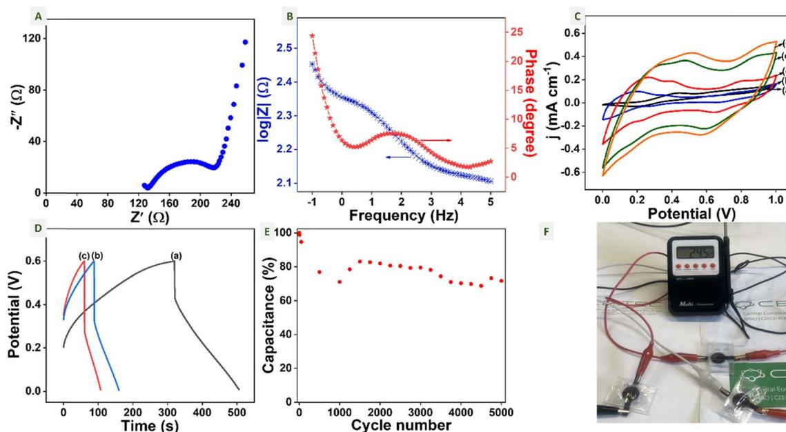
Fig. 6 Electrochemical performance studies of TC-3DE supercapacitors: (A) Nyquist plot, (B) Bode plot, (C) cyclic voltammograms at different scan rates ((a) 1, (b) 5, (c) 25, (d) 75, and (e) 100  $\text{mV s}^{-1}$ ), (D) GCD curves of the symmetric TC-3DE cell at different current densities ((a) 150, (b) 200 and (c) 250  $\text{mA g}^{-1}$ ), (E) cycling stability of the symmetric TC-3DE cell and (F) photograph of a timer being powered using TC-3DE cells.
