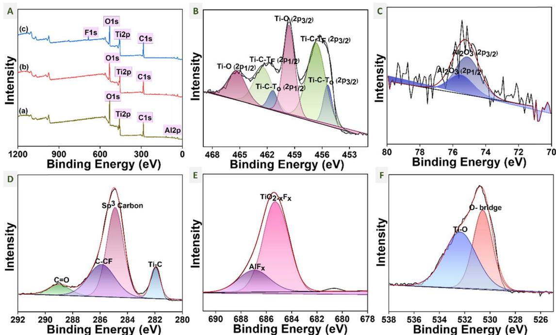
Fig. 4 Elemental composition of MSTC-OX: (A) XPS wide energy spectra of  $\text{Ti}_3\text{AlC}_2$ , MSTC-00 and MSTC-OX (down to up). High resolution elemental (B) Ti 2p, (C) Al 2p, (D) C 1s, (E) F 1s, and (F) O 1s spectra of MSTC-OX.
