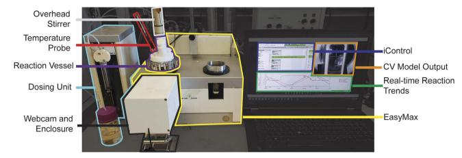
Fig. 2 Experimental workflow setup of *HeinSight 2.0*, illustrating the integration of EasyMax hardware components (dosing unit, overhead stirrer, temperature probe, and reaction vessel), webcam (within an enclosure), and software components ((CV model and iControl) with real-time trend visualization).
