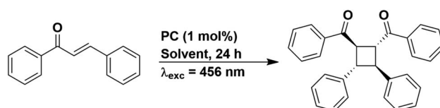
Fig. 11 Reaction scheme for the [2 + 2] cycloaddition of trans -chalcone.
