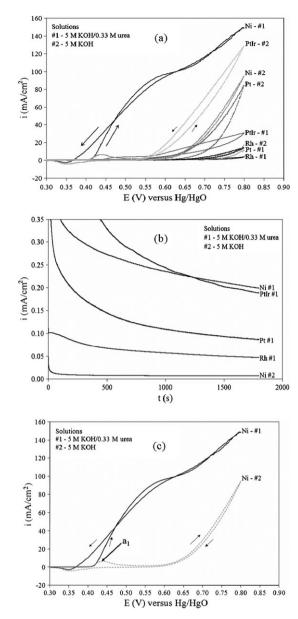
Fig. 2 Anode catalyst analysis at 25 °C: (a) cyclic voltammograms obtained in 5 M KOH with and without the presence of urea on Ti-foil supported electrodes with a 10 mV s<sup>-1</sup> scan; (b) constant voltage test with 1.4 V potential step with 5 M KOH–0.33 M urea; (c) cyclic voltammogram of Ni/Ti electrode in the absence (grey) and presence (black) of 0.33 M KOH in 5 M KOH solution.
