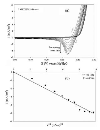
Fig. 3 (a) Cyclic voltammograms obtained in 5 M KOH + 0.33 M urea for the NOMN electrode with various scan rates ( $\nu$ ) from 5 mV s<sup>-1</sup> to 95 mV s<sup>-1</sup>. (b) The plot of cathodic current density variation with  $\nu^{1/2}$ .
