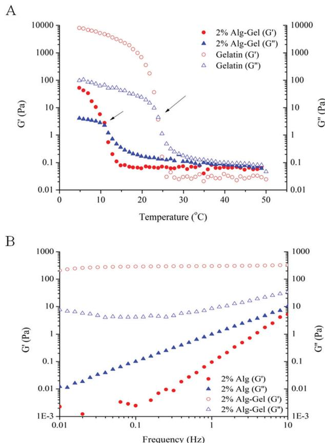
**Fig. 2** Rheological measurements. (A) Temperature sweep measurements comparing Alg-Gel with gelatin. Gelation temperature indicated by the temperature where  $G'$  intersects  $G''$  (indicated by arrows); (B) frequency sweep measurements comparing 2% Alg to 2% Alg-Gel.
