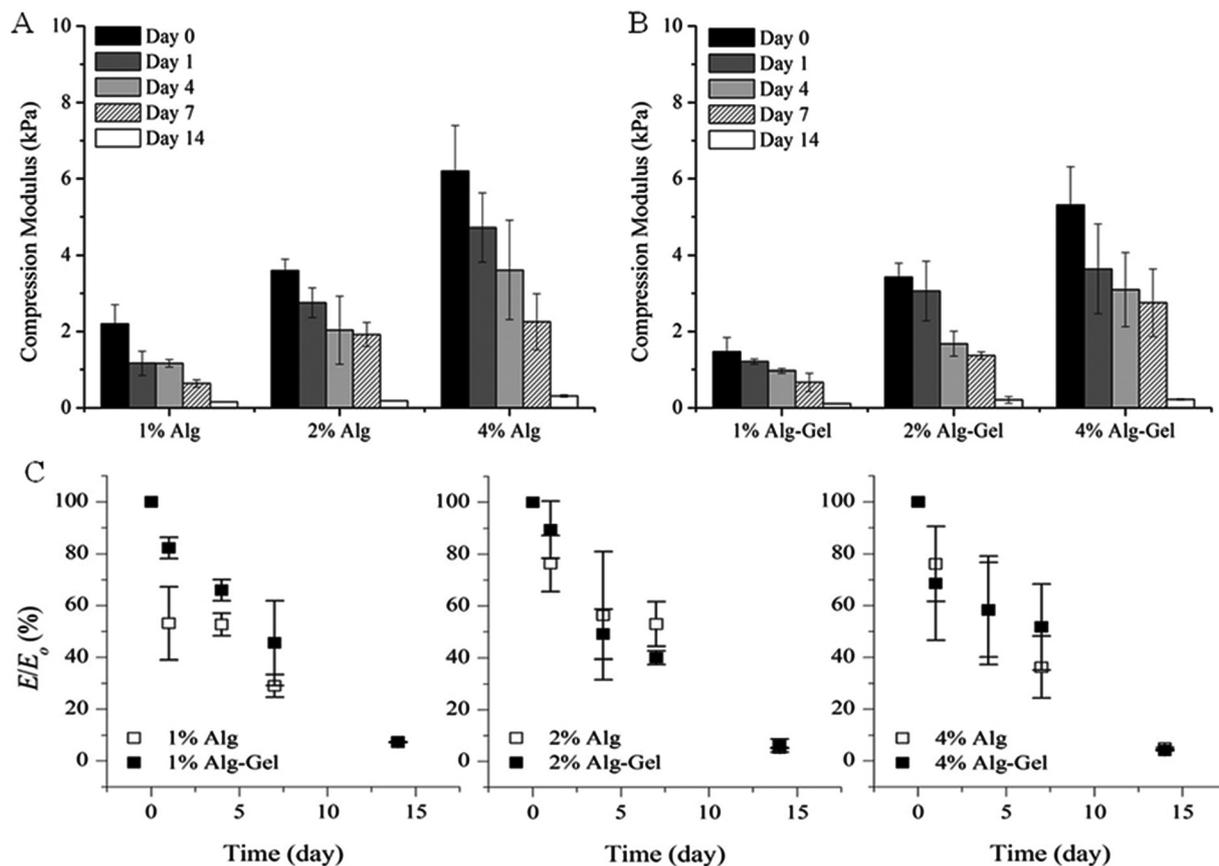
**Fig. 7** Compression modulus of (A) Alg; and (B) Alg-Gel in cell culture medium over 14 days. (C) Modulus remaining. Expressed as a percentage of the modulus ( $E/E_0$ ) at the specified time point relative to the initial modulus at day 0. Data represents mean  $\pm$  s.d.
